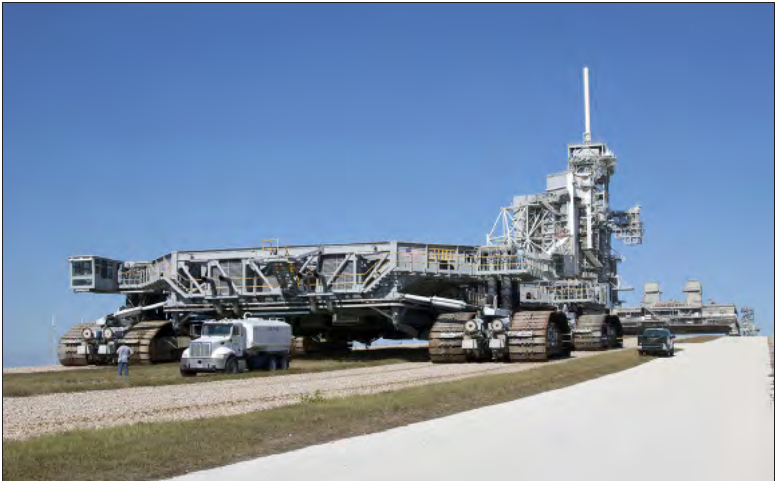
Crawler-transporter 1 approaches the top of Launch Pad 39A after traveling along the crawlerway at Kennedy Space Center on Dec. 3. New jacking, equalizing and leveling, or JEL, hydraulic cylinders were installed on CT-1 and are undergoing a leveling and turning test as the crawler travels along the slope. Photo credit: NASA/Daniel Casper
