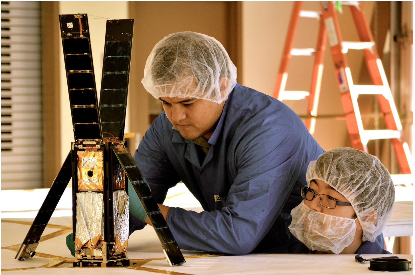
LightSail team members Alex Diaz (left) and Riki Munakata (right) prepare the spacecraft for a sail deployment test. Credit: The Planetary Society.
