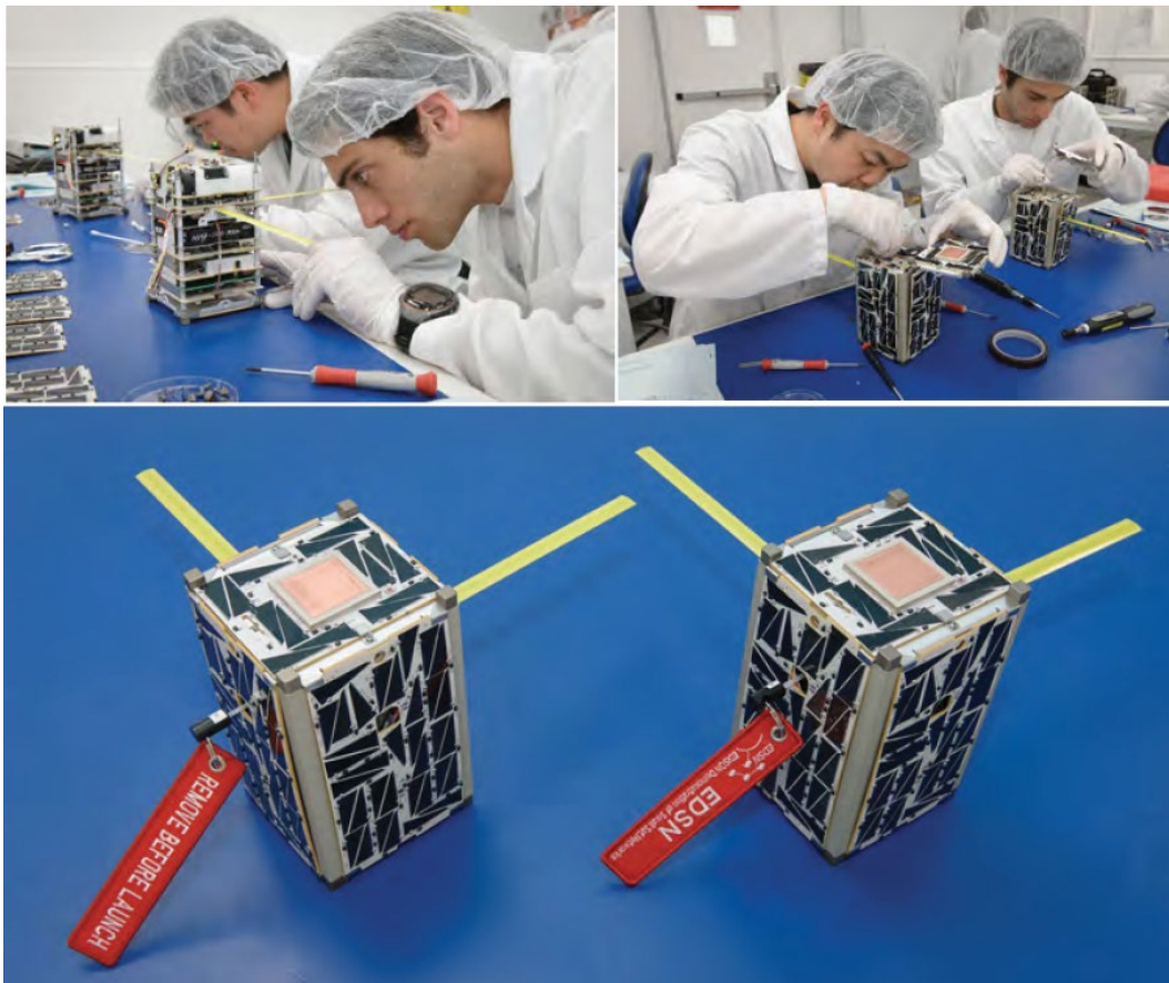
EDSN Spacecraft Assembly Sequence (top) and Completed EDSN Spacecraft (bottom)
