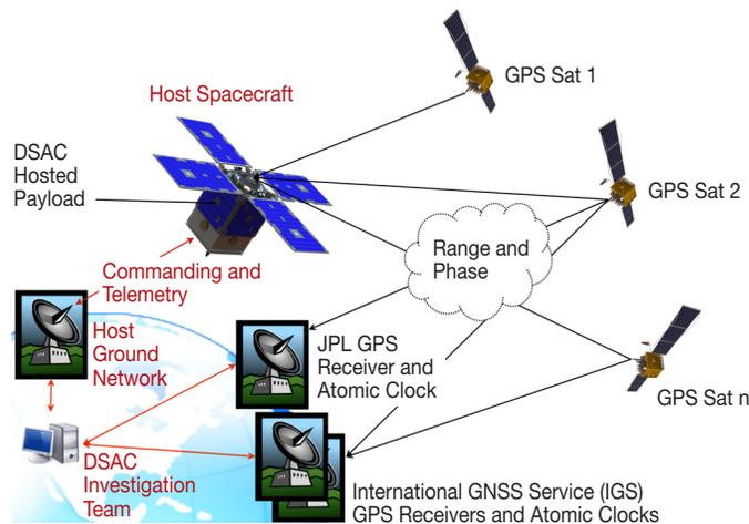
Figure 3. DSAC on-orbit demonstration mission architecture.
