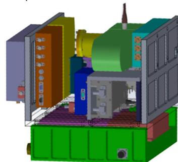
Figure 2. Preliminary design of DSAC with the outer cover removed, showing the internal components.
