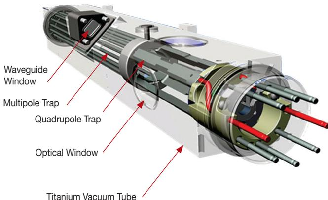
Figure 1. Drawing of the DSAC mercury-ion trap showing the traps and the titanium vacuum tube that confine the ions. The quadrupole trap is where the hyperfine transition is optically measured and the multipole trap is where the ions are "interrogated" by a microwave signal via a waveguide from the quartz oscillator.
