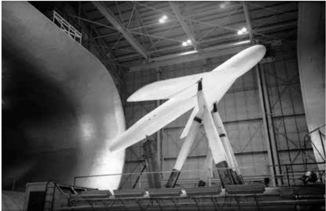
Following these initial results, suction slots were relocated near the wing leading edge, and the test program focused on the control of leading-edge separation by suction.<sup>14</sup> The slots were located at the 0.015- and the 0.025-chord stations, where the concept was much more effective. In the 1940s, this fundamental information was largely unknown, and the data gathered in the study helped form the foundation for evolving boundary-layer control concepts.
