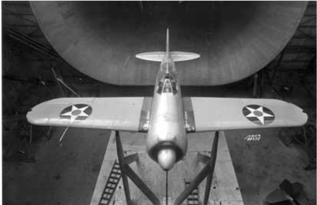
The XF2A-2 remained at Langley and was again tested in the Full-Scale Tunnel a few months later in April 1941 at the request of the Navy, to determine the effects of wing-mounted machine-gun and cannon installation configurations on maximum lift and drag.<sup>27</sup> Results showed that, for minimal impact on lift, the ends of the machine guns should be flush with the leading edge of the wing rather than protruding and that cannons carried in underwing gondolas caused excessive drag.
