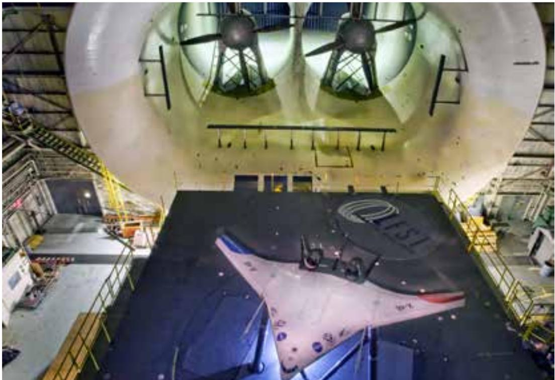
cooperative Boeing and NASA ground-based acoustic research, the X-48B configuration was modified to further enhance the reduced-noise potential of the BWB configuration. The modifications included removal of the winglets and the addition of noise-shielding twin vertical tails with rudders, replacement of the original three turbojet engines with two larger fanjet engines, and an extended deck area.
