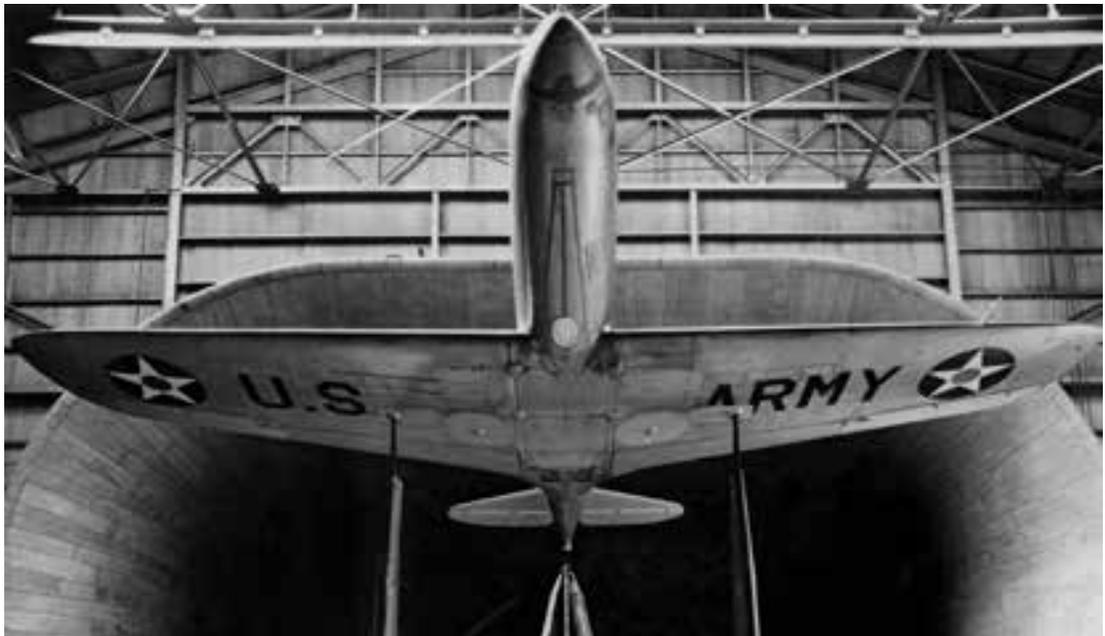
reduce the drag contribution by 50 percent. Finally, it was recommended that the landing gear design be modified to produce a flush wing and fuselage surface when retracted.
