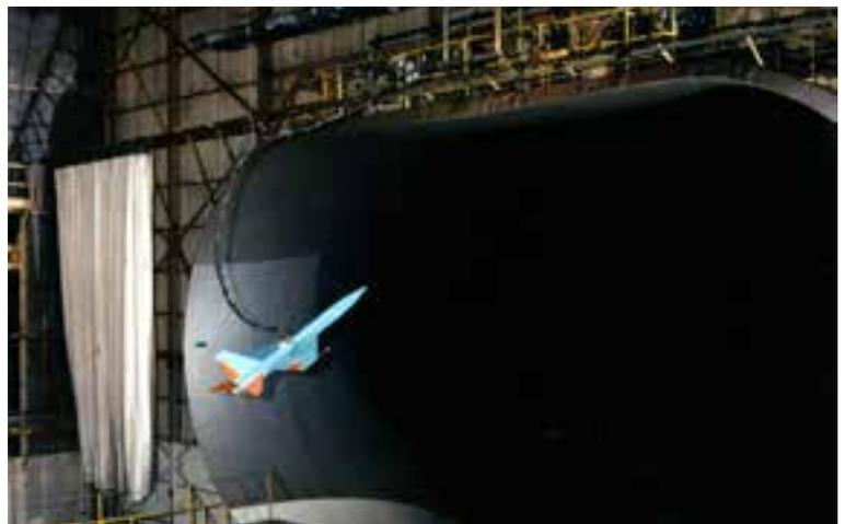
model tests for the first-ever flight demonstration of the integrated control system used a generic fighter configuration equipped with conventional, thrust-vectoring, and pneumatic-forebody controls. The free-flight model computer used at the Full-Scale Tunnel was programmed with appropriate control laws, and the effectiveness of pneumatic forebody controls was demonstrated without the use of rudders or thrust vectoring for additional yaw control.<sup>17</sup>
