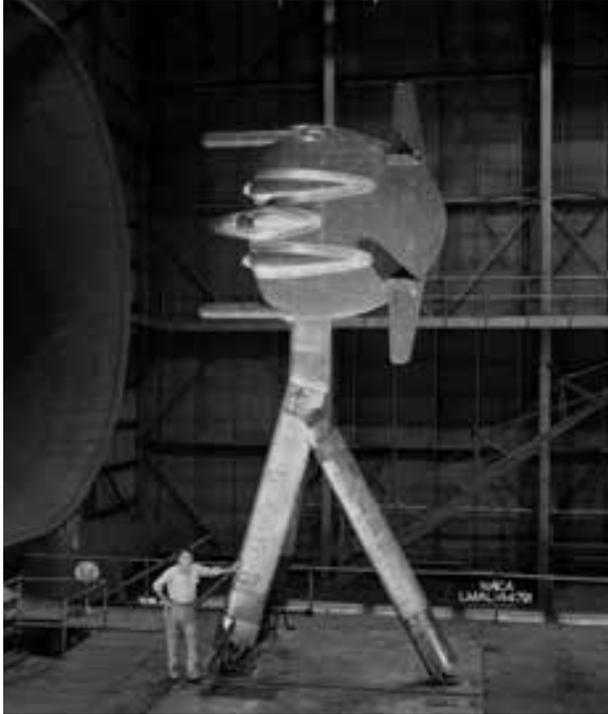
rather than downward in the center. Although the data obtained in the tests were sufficient to determine the propulsive characteristics, effective propeller operation, and static thrust of the propellers, the test program was terminated prematurely by the failure and complete destruction of one of the model's propellers.
