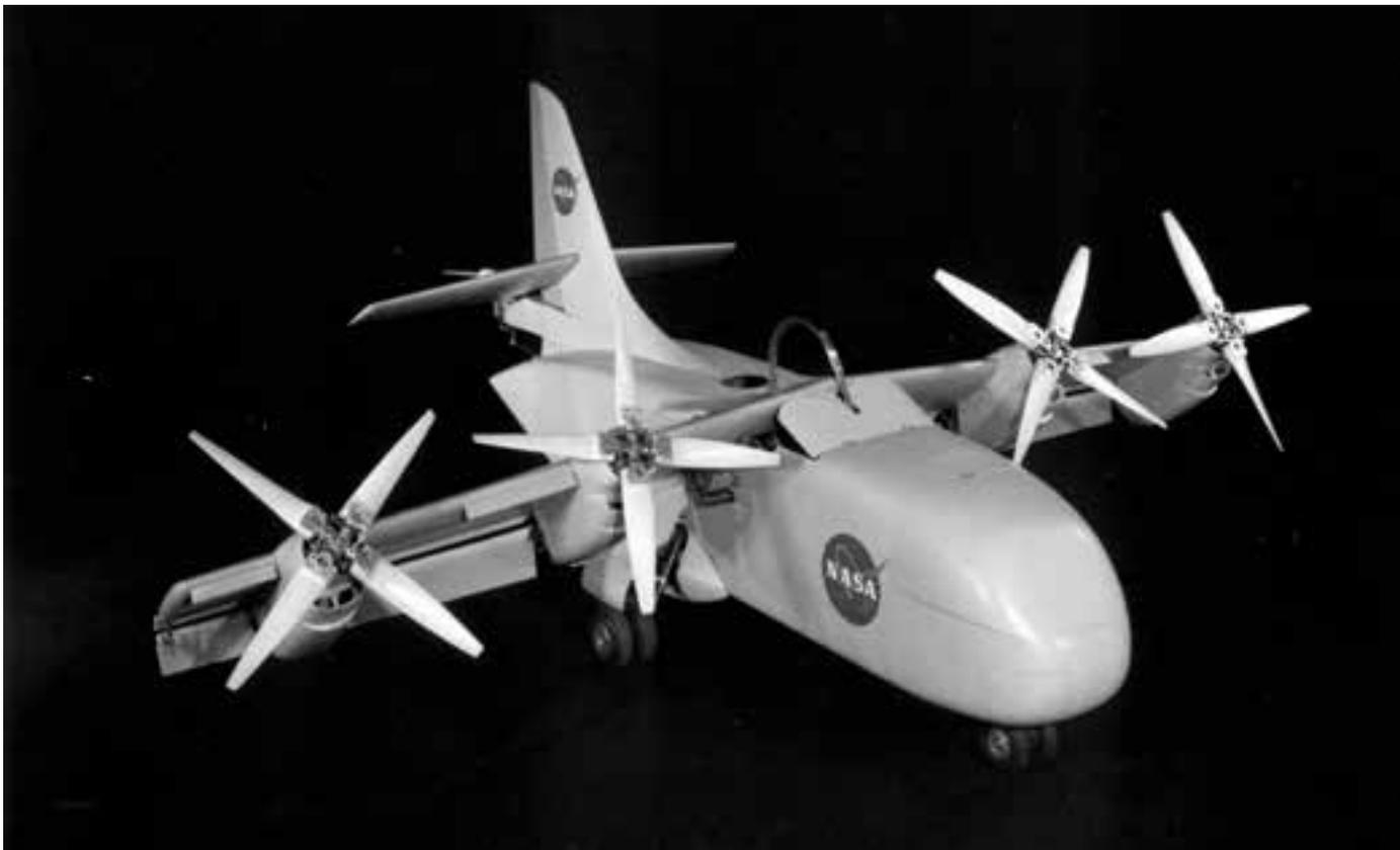
the XC-142A was provided by differential deflections of the propeller blade pitch of the four main propellers; yaw control was provided by differentially deflecting the ailerons; and pitch control was provided by varying the pitch of the tail-mounted rotor. These control functions were phased out as the transition to forward flight progressed, resulting in the use of conventional control surfaces.)
