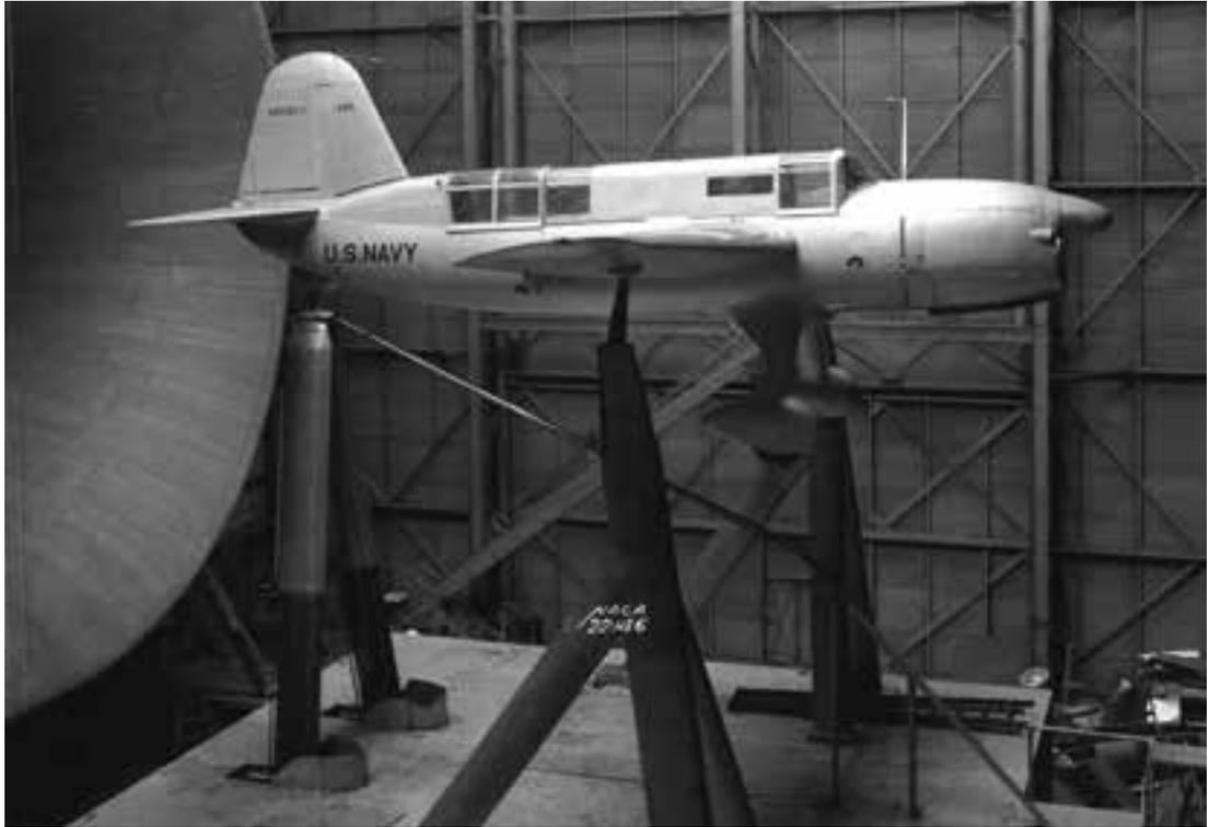
At the Navy's request, an investigation of the cooling and stability problems of the XSO3C-1 was made in the Full-Scale Tunnel in October 1940.<sup>59</sup> The tests included extensive power-on and power-off thermocouple measurements of the cooling behavior both in the baseline condition as well as with an improved cowling inlet, cylinder baffles, and cowling outlets. At the end of the program, a few traditional drag cleanup tests were conducted.
