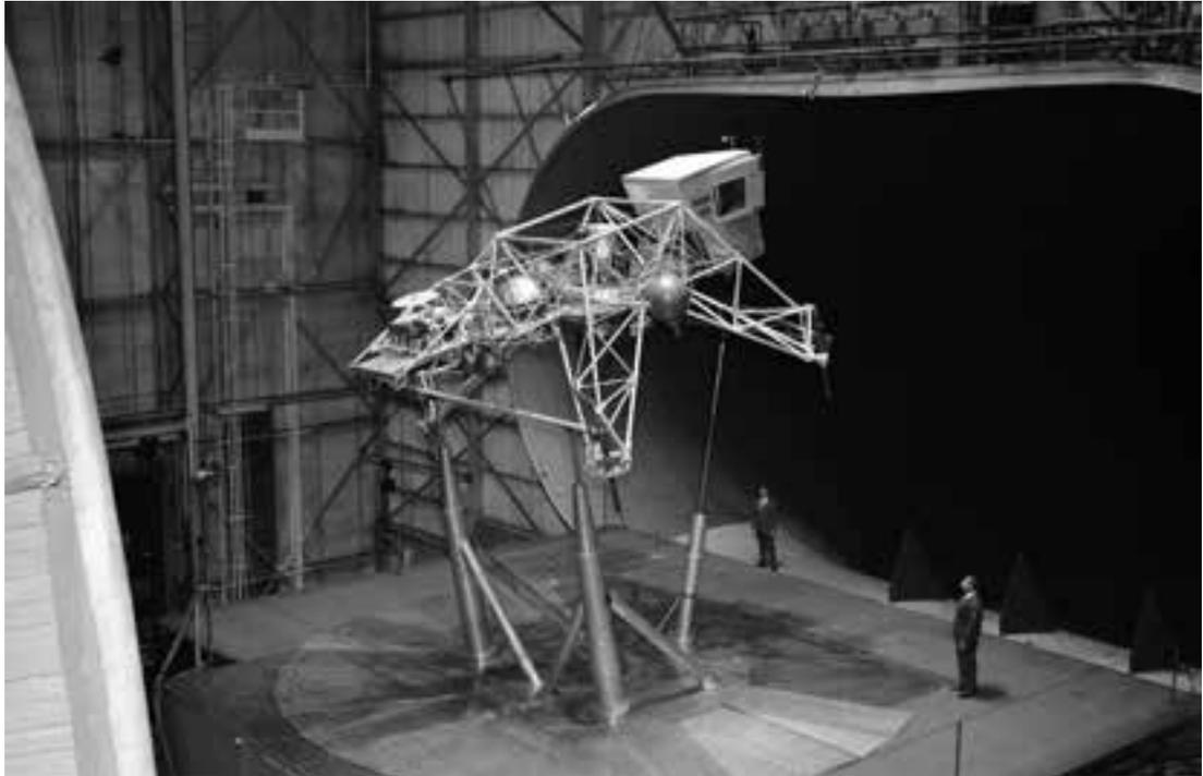
required had exceeded the ability of the yaw thrusters to control the vehicle. The ensuing accident investigation board recommended that another LLTV be tested in the NASA Langley Full-Scale Tunnel to investigate the aerodynamic behavior and controllability of the configuration. Accordingly, LLTV 3 was loaded aboard a modified Boeing Stratocruiser “Super Guppy” and flown to Langley for installation in the tunnel.
