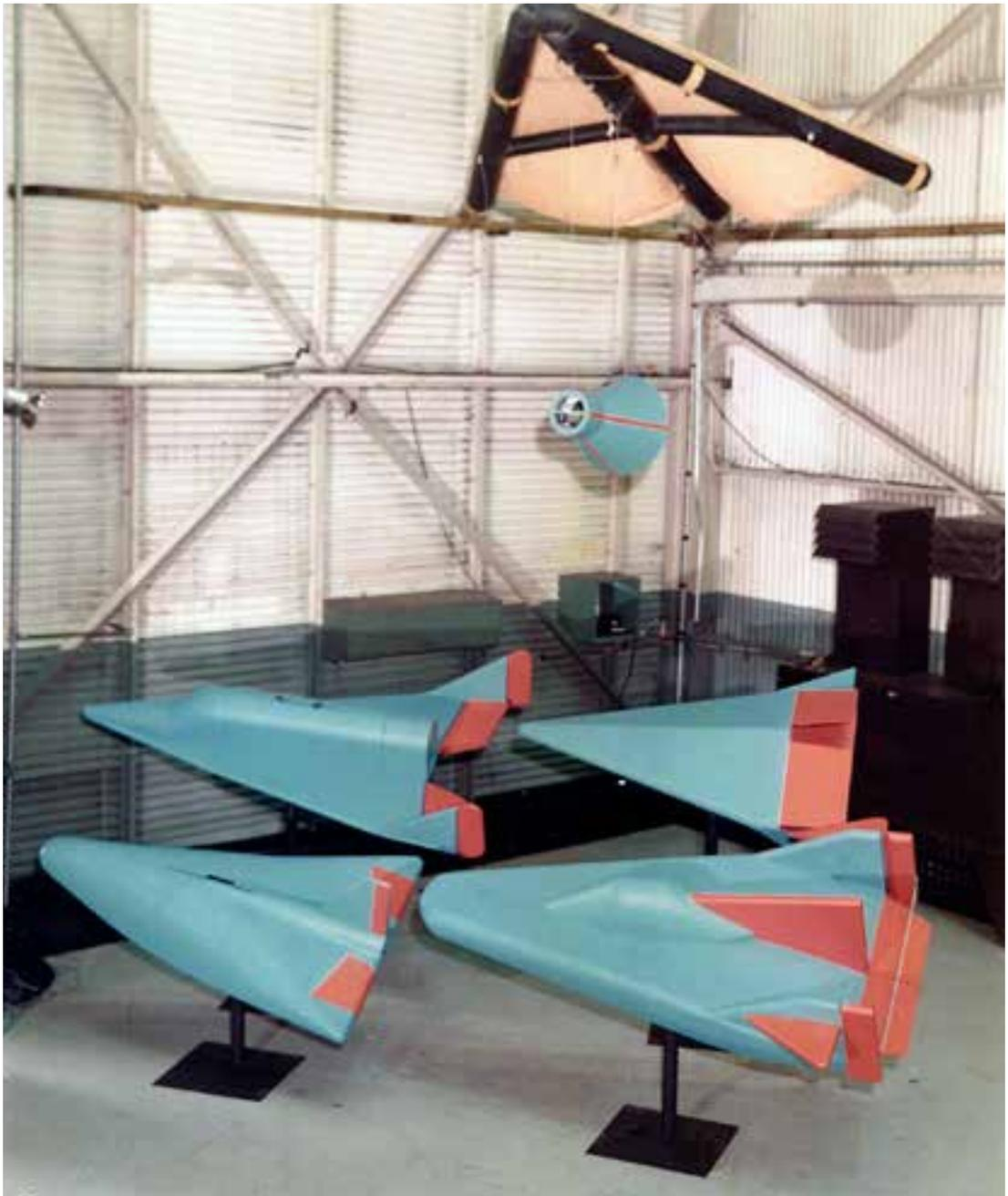
than 10 different HL-10 models in various wind tunnels—over 8,000 hours of tunnel testing were involved.<sup>29</sup>
