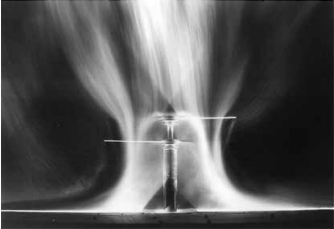
observed, and the starting vortex associated with the sudden increase in thrust was easily observed as well. The balsa-dust technique has been noted as a particularly valuable contribution to rotorcraft technology.<sup>21</sup>
