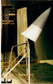
The F-15 radome test was a combined effort, with participation by ODU, Bihrl Applied Research, and the Air Force. Production radomes were used in the tests, which included extensive pressure,
