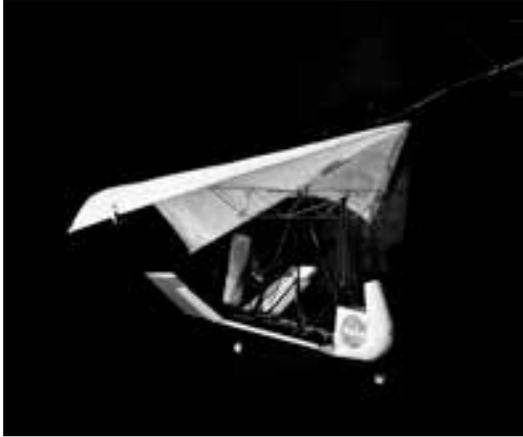
Jeep). Although the Fleep vaguely resembled the Flex-Wing, it included several changes to correct deficiencies exhibited by the previous design. The wing-banking and pitching concept that had resulted in unsatisfactory roll control of the Flex-Wing was replaced by a system similar to the one devised by the staff at the Full-Scale Tunnel.
