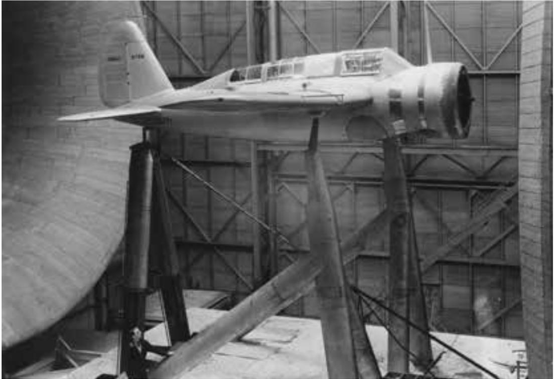
airplane was also found to have excellent stall characteristics and, for the highest angle of attack tested, the wing leading edge, the wingtips, and a portion of the ailerons were still not stalled. The analysis of rudder forces indicated a poor tail mechanical design, and a floating rudder tab was recommended along with an increase in size of the vertical tail.
