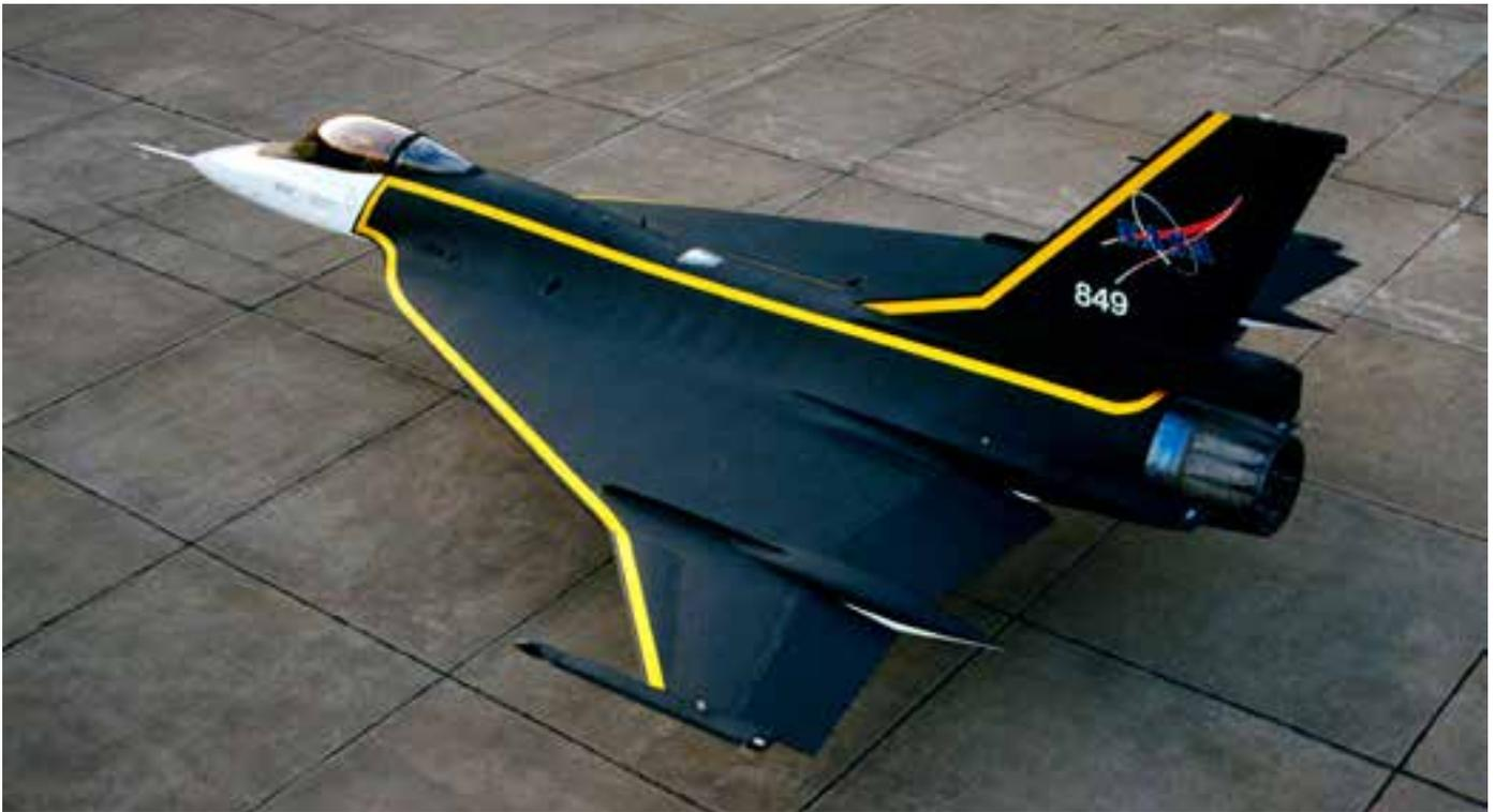
moderate angles of attack. In particular, the objective of the investigation was to maximize lift-to-drag ratio while reducing nose-up pitching moments. The model featured a cranked-delta wing and inboard- and outboard-leading-edge flap segments.<sup>24</sup>
