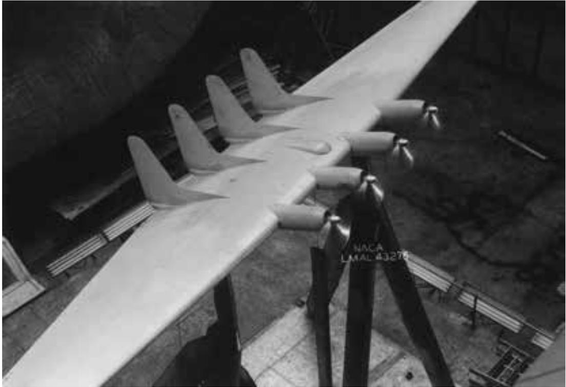
survey analysis). The data indicated that the model was longitudinally, laterally, and directionally stable for most conditions, but as expected, the rudder effectiveness and directional stability of the model were much lower than those of conventional aircraft. The aerodynamic results of the tests were used in a brief analysis of the flying qualities of the airplane.<sup>135</sup>
