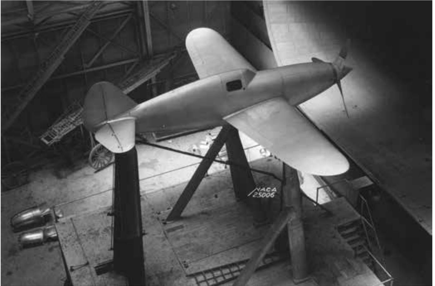
measurements of longitudinal stability and control, including the effects of wing flaps and propeller slipstream. Stick-force characteristics and the contributions of tail components and stability are also determined.
