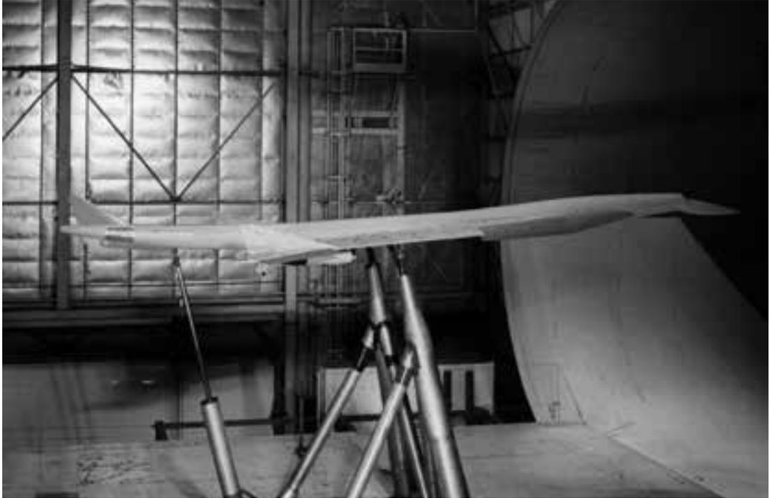
Tunnel were used for noise studies, and acoustic testing was not pursued in the Full-Scale Tunnel after the 1970s. The acoustic treatment remained in place within the tunnel's test section for the remaining life of the facility.
