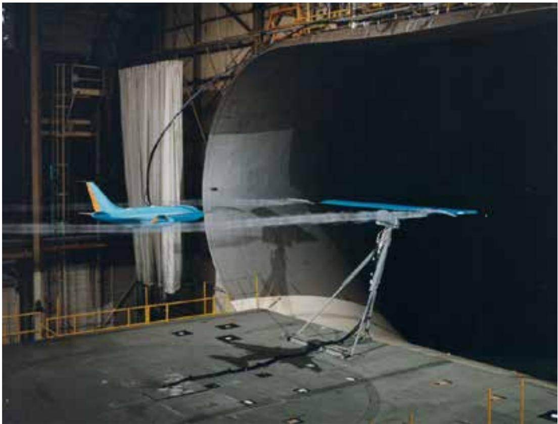
static test setup in which the magnitudes of the forces and moments induced by the trailing vortex were measured on a sting-mounted model.<sup>36</sup> A vortex-generating wing was mounted to the movable tunnel survey carriage upstream of the test model and was positioned at various locations to map the effects of the vortex on the downstream model. A five-hole survey probe was also used to quantify the wake-velocity characteristics at the model's position.
