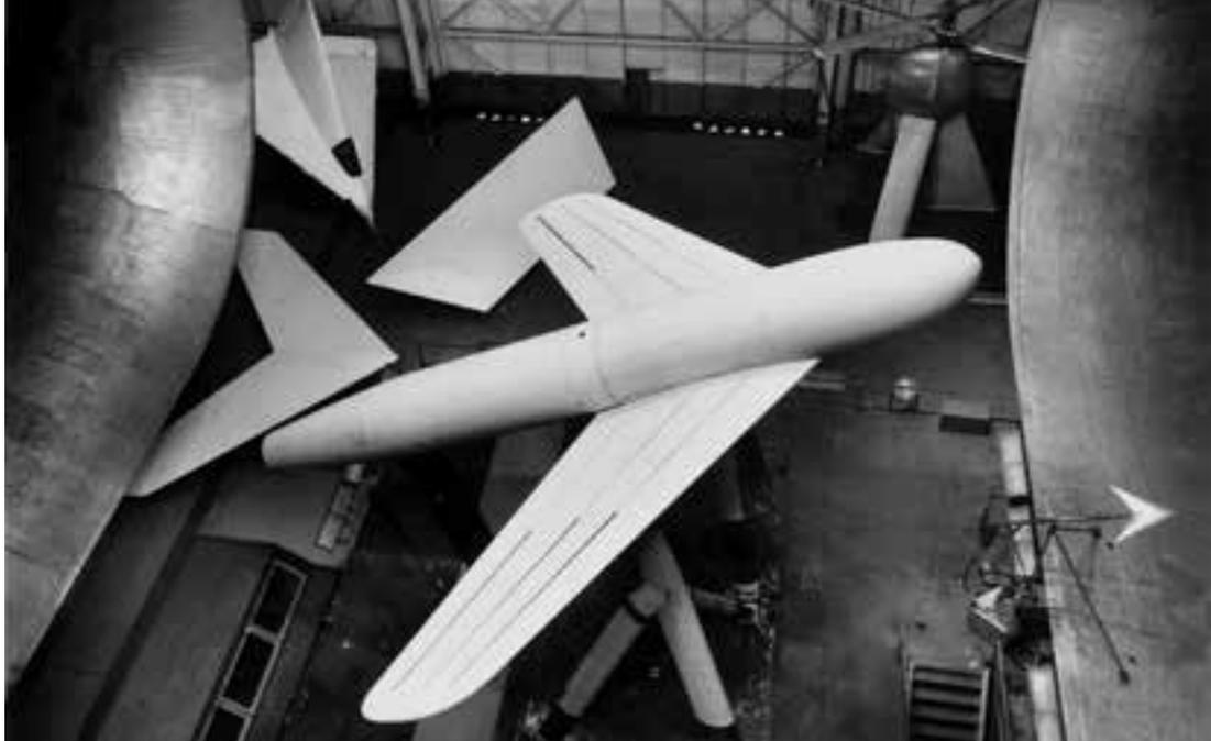
A large number of test subjects were evaluated over several years in the late 1940s, including swept wings, rectangular wings, delta wings, wings with pointed tips, and cranked wings with different inboard and outboard sweep angles.<sup>12</sup> All the models included relatively sharp
