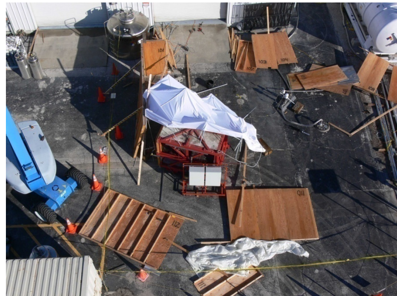
Area surrounding test unit following tank rupture. Test team location was behind roll-up door at top of image.
