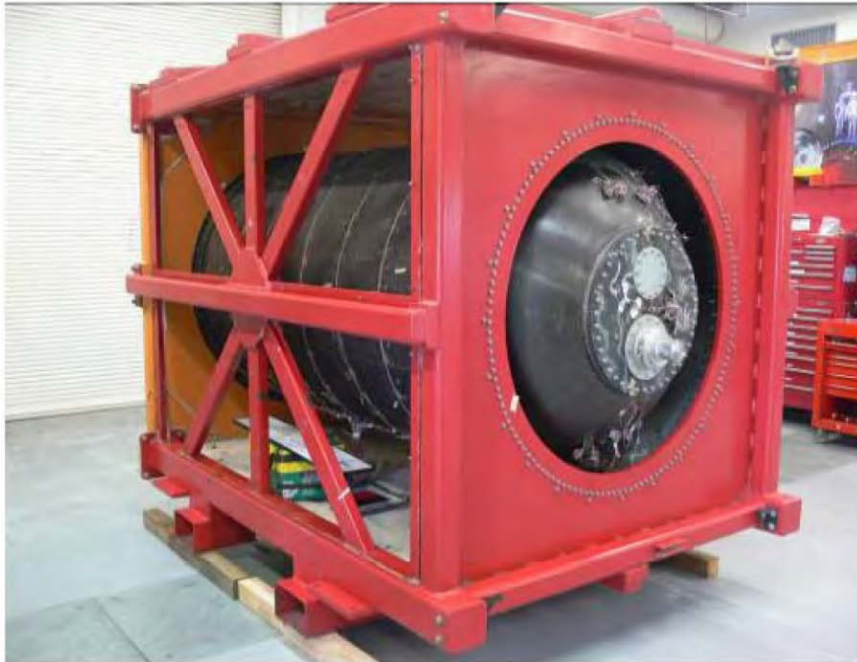
Figure 2-2. Composite Tank in Support Structure
