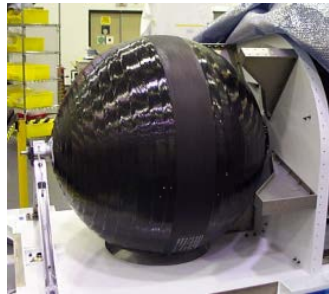
High Pressure Gas Tank (HPGT) – Oxygen COPV (37.89"D)
