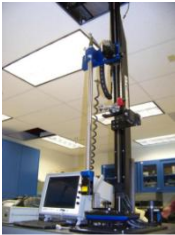
External Profilometer added to Original Scanner
