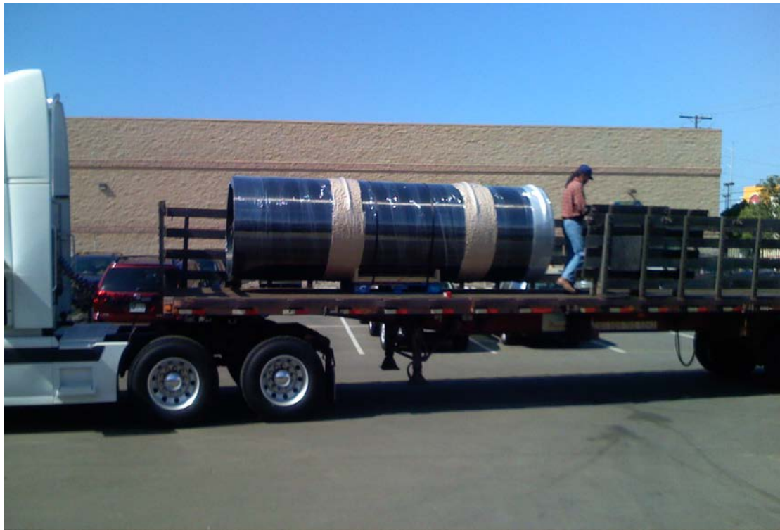
Local transport of a 200 cu. ft. 500 psi LOX tank
