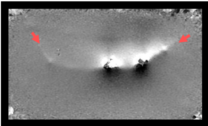
Shearography image showing debonding of metal liner from composite over wrap.
