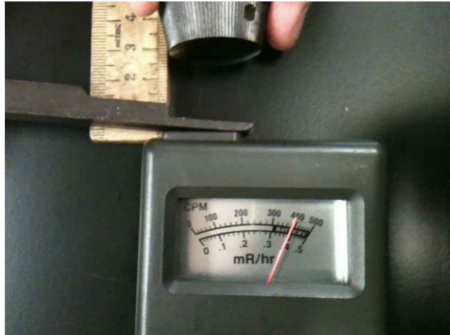
Geiger counter used for testing gamma and x-ray exposure
