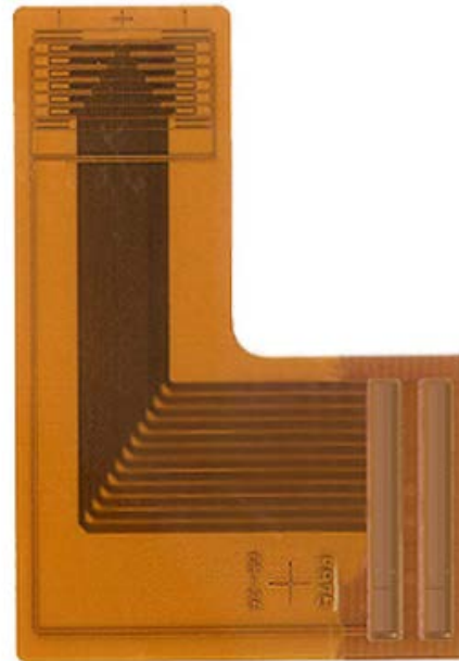
Room Temperature MWM-Array Sensor
