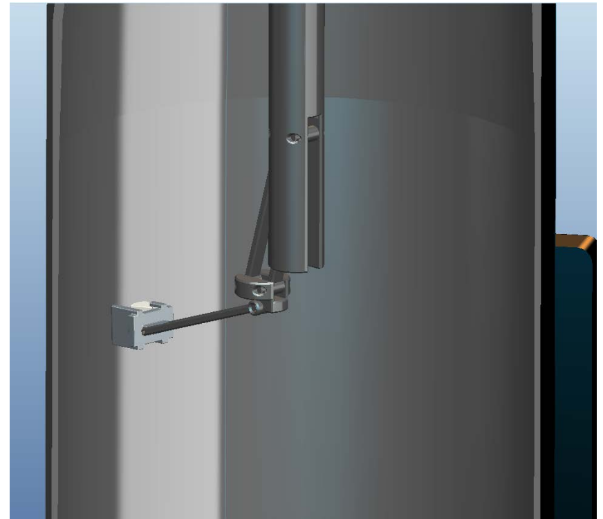
Collapsible internal EC probe deployed for scans (conceptual design)
