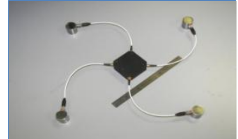
DIDS system with sensors and short cables
