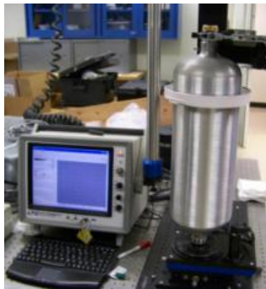
External Eddy Current (EC) Probe added
