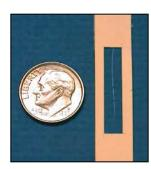
Single glass filaments are used for strength, elongation and modulus measurements
