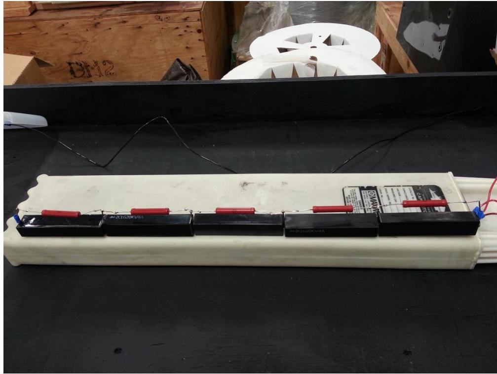
**Figure 26 – 100kV diode bridge and test capacitor.**
