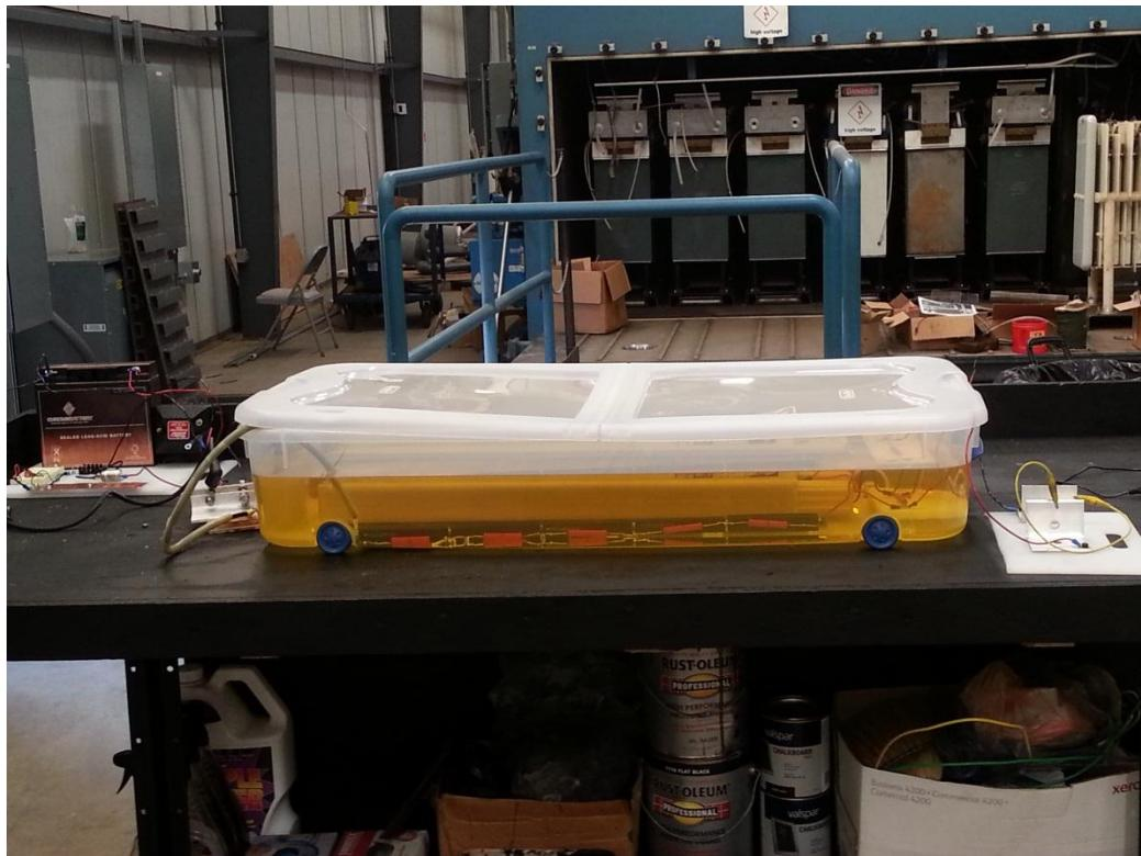
**Figure 29 – 1kJ Pulser ready for test.**
