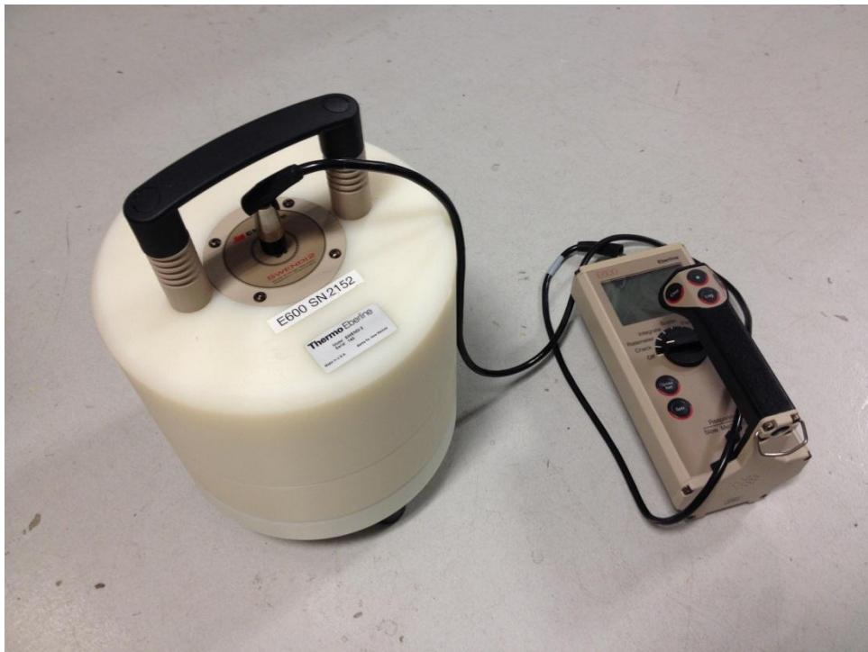
**Figure 43 - Thermo Eberline SWENDI 2 neutron probe with counter.**
