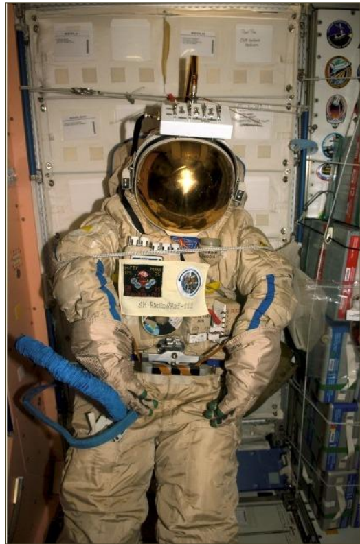
SuitSat-1 created using a decommissioned Russian Orlan spacesuit that is outfitted with transmission hardware will be released by hand during an EVA. NASA image ISS012E15666
