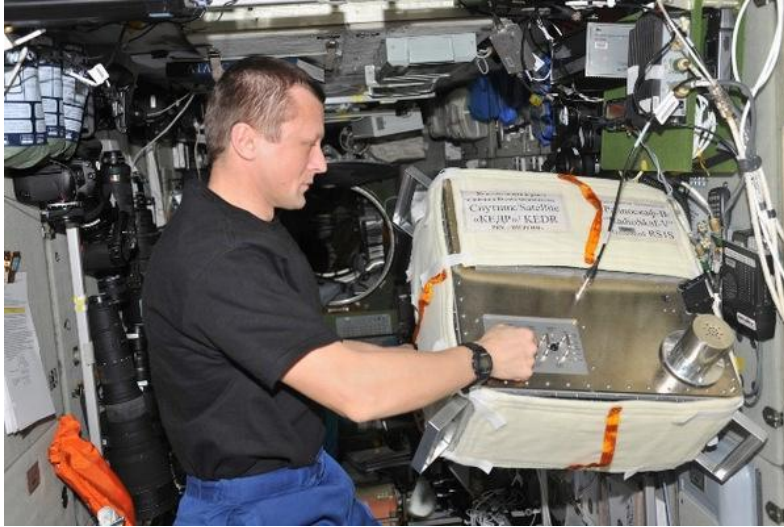
Russian cosmonaut Dmitri Kondrat'ev (onboard engineer on Expedition 26/27) performs a test checkout of the satellite ARISSat-1/Kedr.
