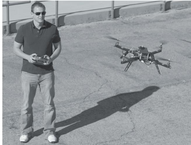
*Dryden researcher Loyd Hook flies the quad rotor research vehicle to validate research on elements of a futuristic control system that has immediate applications for unmanned aircraft systems and potentially to a future personal air vehicle.*
