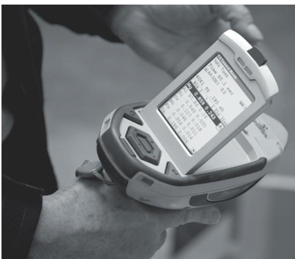
*This material analyzer is one of the most recent tools used to uncover substandard materials and counterfeit parts.*
