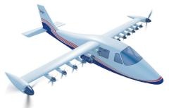
When complete, the X-57 Maxwell test program hopes to have demonstrated how to safely operate an all-electric, zero-emissions aircraft, including its battery and power distribution systems. That knowledge will be helpful to future engineers interested in designing all-electric air vehicles that might be used for everything from urban air mobility to moving passengers and cargo between nearby cities.
