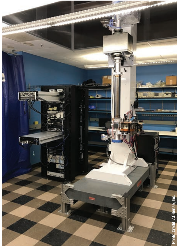
The Goddard-AOSense team built this terrestrial proof-of-concept gravity gradiometer.
