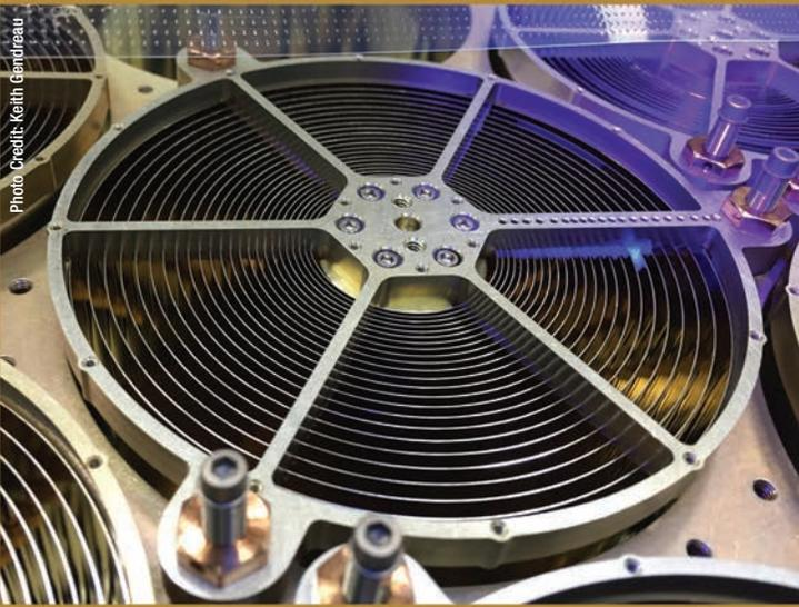
This is a closeup of one of the 52 X-ray mirror assemblies on NICER. These mirror assemblies concentrate X-rays onto silicon detectors to gather data that probes the interior makeup of neutron stars, including those that appear to flash regularly, called pulsars.
