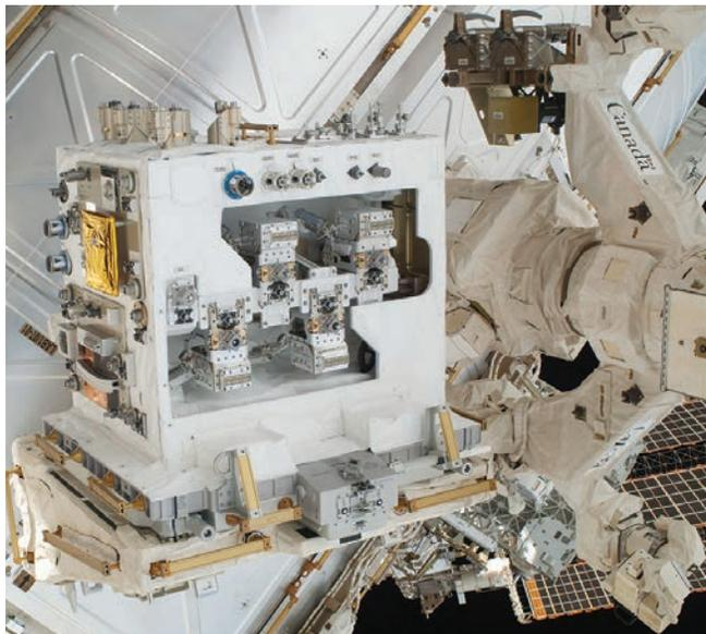
*The Robotic Refueling Mission, or RRM, module was temporarily installed on the Dextre robot's Enhanced ORU Temporary Platform on the International Space Station. RRM resided there for nearly two months before being transferred to its permanent location on an external platform fit for its robotic demonstrations.*
