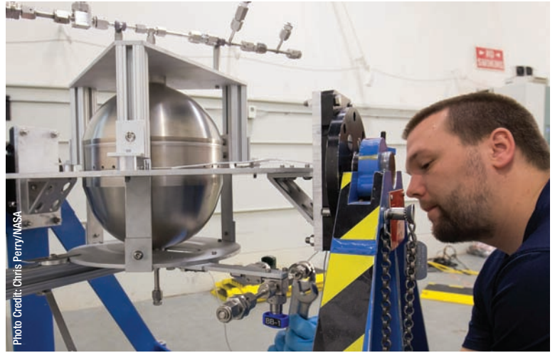
This image shows the tank that held the Swedish-developed green propellant. Kyle Bentley is pictured.
