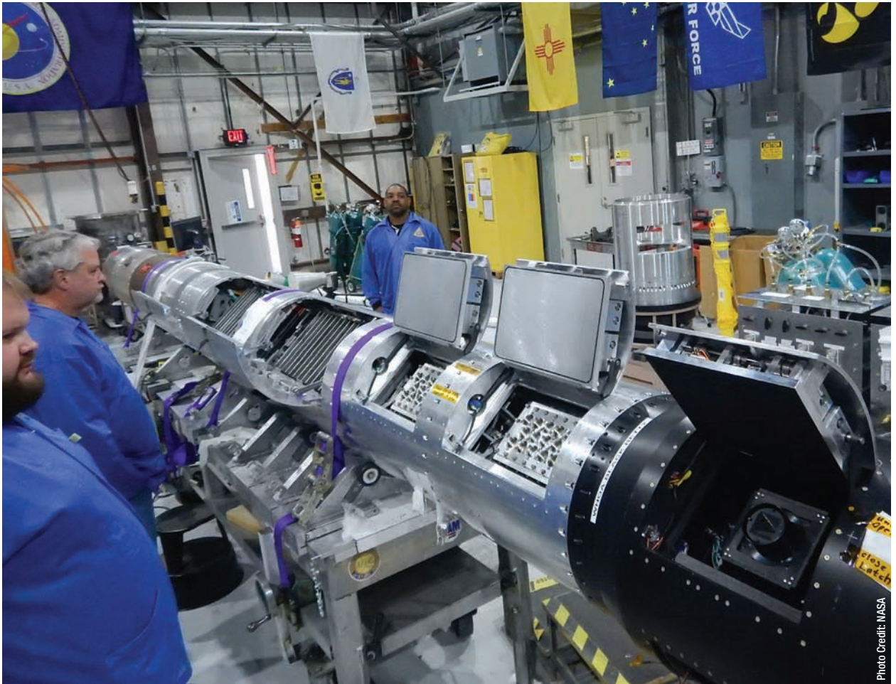
The CuPID/WASP payload (front of rocket) was integrated into a Black Brant IX sounding rocket and launched in early December 2015. The instrument returned valuable data needed by three different scientific disciplines.
