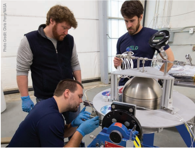
A Goddard team, led by engineer Henry Mulkey (middle), prepares a tank containing a Swedish-developed green propellant before its simulated loading at the Wallops Flight Facility late last year. Kyle Bentley (squatting) and Joe Miller (standing to the right of Mulkey) assisted in the demonstration.
