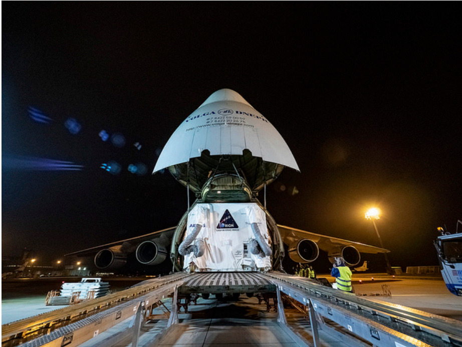
Nov 5 - Bremen, Germany. Orion's European Service Module is loaded on the Antonov airplane for transport to Kennedy Space Center.
