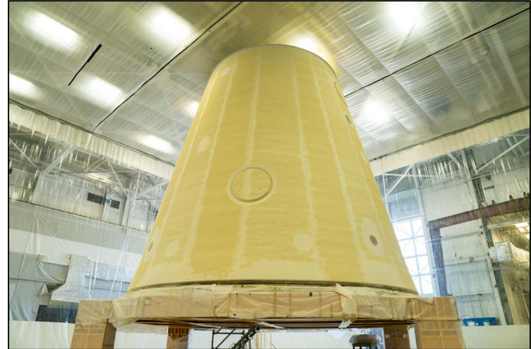
Thermal Insulation Application Complete on LVSA
