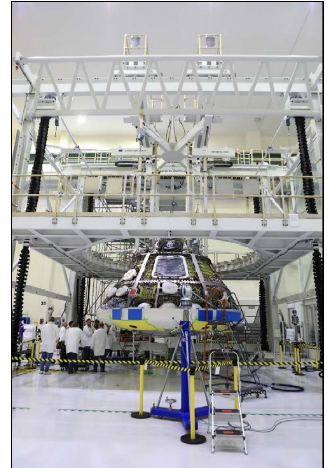
EM-1 Heat Shield Installation at KSC
