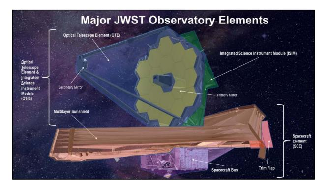
There are two primary elements of the JWST observatory. The first is the combined <u>Optical Telescope</u> Element and <u>Integrated Science Module</u>, or OTIS. The second is the Spacecraft Element (SCE), which is the combined Spacecraft Bus, Trim Flap, and Multilayer Sunshield.
