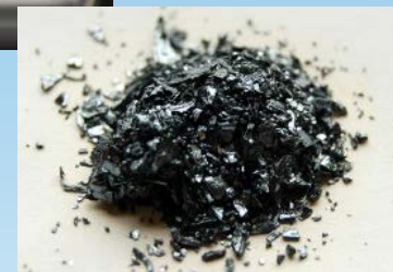
300cc Iodine Propellant Stored as Solid Crystals
