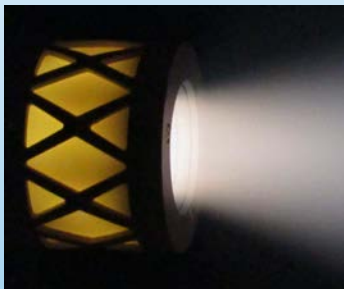
Busek 3cm RF Ion Thruster BIT-3; 50W Nominal at Thruster Head
