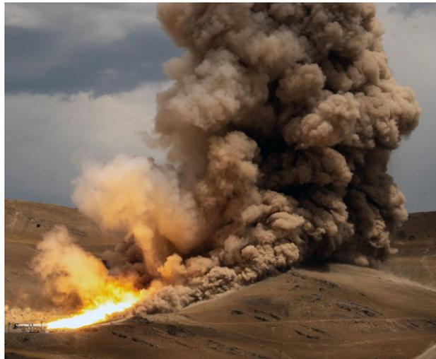
Solid rocket booster motor ground test for future flights of the agency's Space Launch System rocket in Promontory, Utah.
