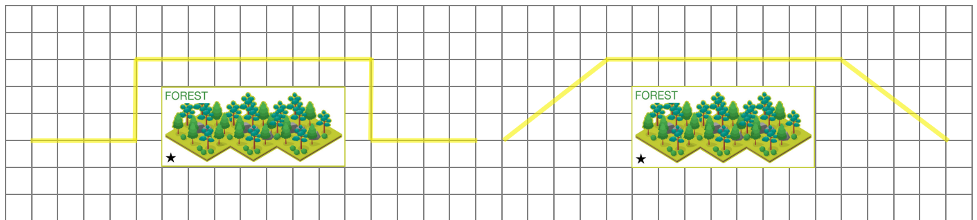
Examples showing UAV flight path turning at grid corners and staying at least 1-unit space away from game piece (obstacle).
