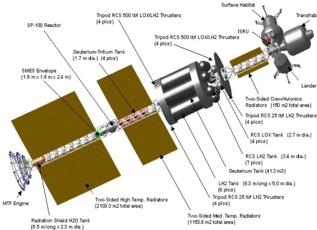
Fig. 4. Layout of the MTF crewed vehicle for a round trip mission to Callisto. Vehicle is self contained with crew transhab, lander, ISRU plant and surface habitat on vehicle.
