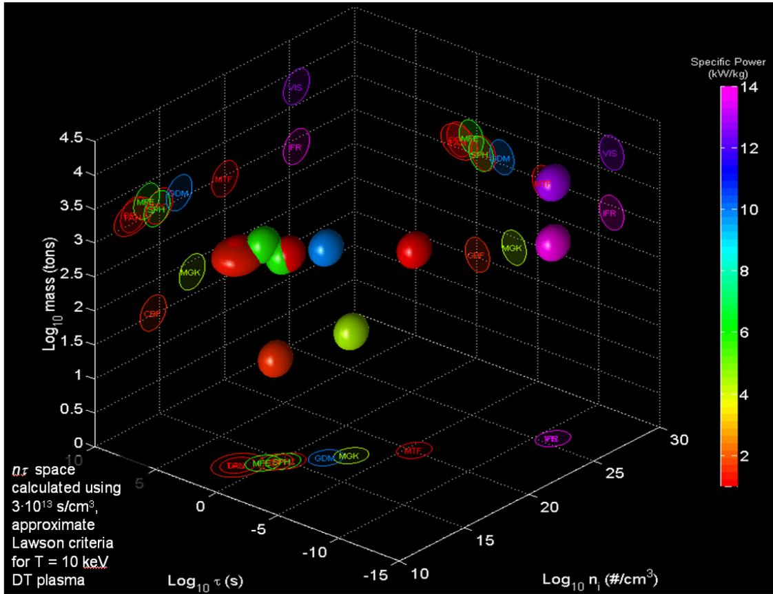
Fig. 1. Map of fusion propulsion concepts in a 4D parameter space of density, confinement time, vehicle mass, and specific power. Performance values can be referenced in Table 1 above. The confinement time is calculated using a Lawson criteria for  $T = 10$ keV DT plasma.
