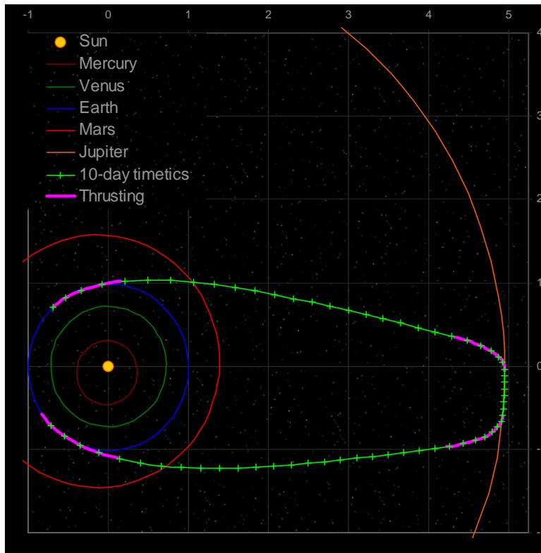
Fig. 3. Trajectory plot of representative crewed mission to Jupiter's moon Callisto using MTF. Pink lines indicate thrusting times and green lines indicate coasting times.
