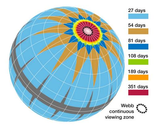
This map illustrates how TESS will cover the sky over its two-year mission. Observation sectors overlap at the ecliptic poles, which are points perpendicular to the plane of Earth's orbit, and provide improved sensitivity there. TESS coverage is maximized within 12 degrees of the ecliptic poles, areas that include zones where the James Webb Space Telescope will be able to observe targets throughout the year. MIT
