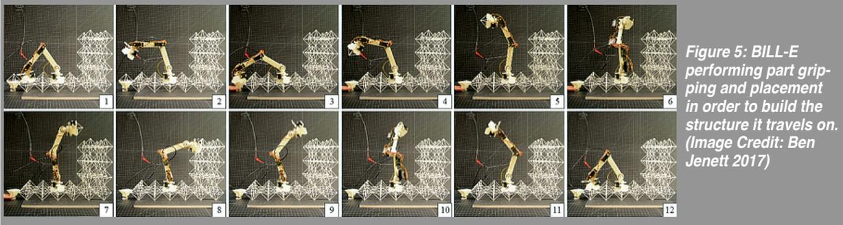
*Figure 5: BILL-E performing part gripping and placement in order to build the structure it travels on. (Image Credit: Ben Jenett 2017)*
