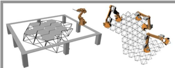
Figure 1: Comparison of robotic assembly platforms for space structures. (left) Traditional motion system with robotic arm, based on work from NASA Langley. (right) Multi-agent relative robotic system (Image Credit: Ben Jenett, 2017)
