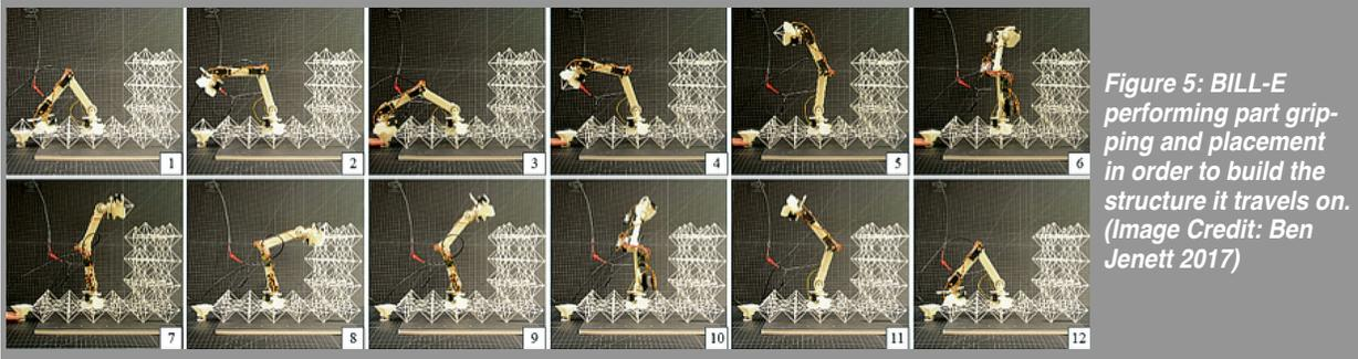
*Figure 5: BILL-E performing part gripping and placement in order to build the structure it travels on. (Image Credit: Ben Jenett 2017)*
