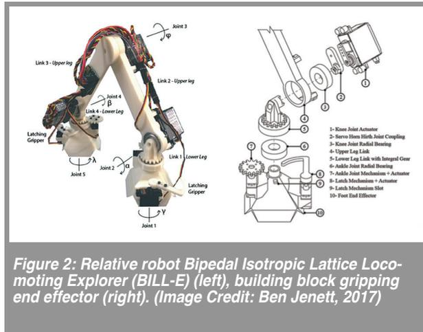
Figure 2: Relative robot Bipedal Isotropic Lattice Locomoting Explorer (BILL-E) (left), building block gripping end effector (right). (Image Credit: Ben Jenett, 2017)
