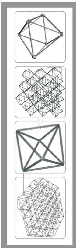
Figure 3: Hierarchical construction of large scale truss structures from building block elements. (Image Credit: Ben Jenett and Christina Gregg, 2017)
