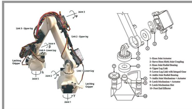
Figure 2: Relative robot Bipedal Isotropic Lattice Locomoting Explorer (BILL-E) (left), building block gripping end effector (right). (Image Credit: Ben Jenett, 2017)
