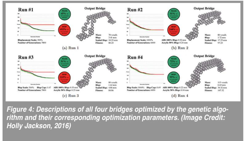
*Figure 4: Descriptions of all four bridges optimized by the genetic algorithm and their corresponding optimization parameters. (Image Credit: Holly Jackson, 2016)*
