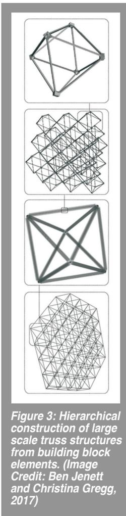
*Figure 3: Hierarchical construction of large scale truss structures from building block elements. (Image Credit: Ben Jenett and Christina Gregg, 2017)*
