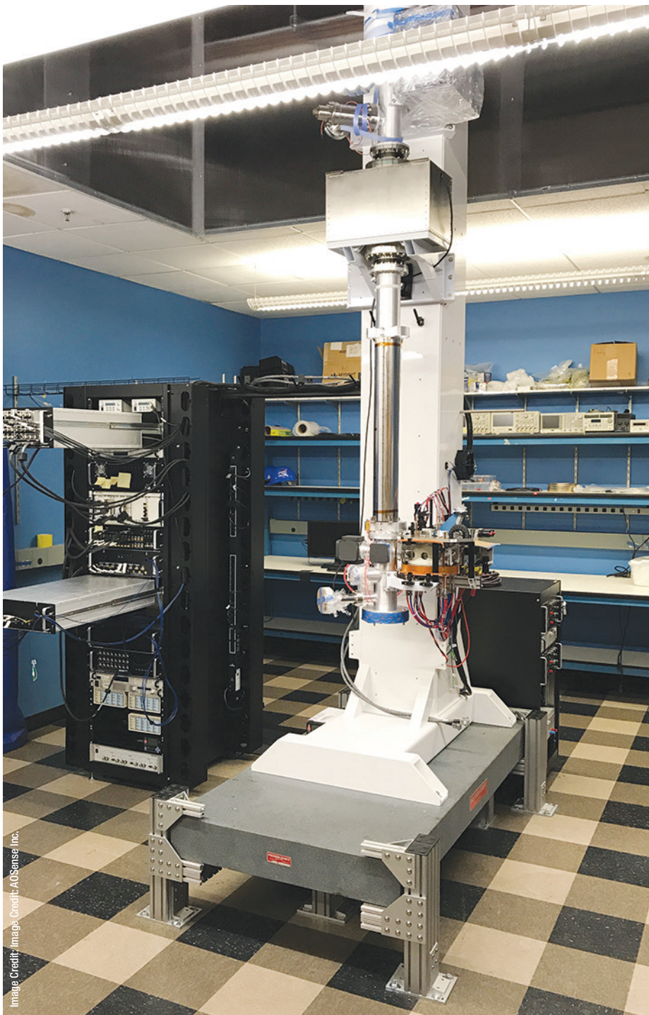
The Atom Interferometer Gravity Gradiometer, shown here at the AOSense Lab in Fremont, California, directly measures changes in gravity's effect on atoms suspended in a cloud at super-cold temperatures.
