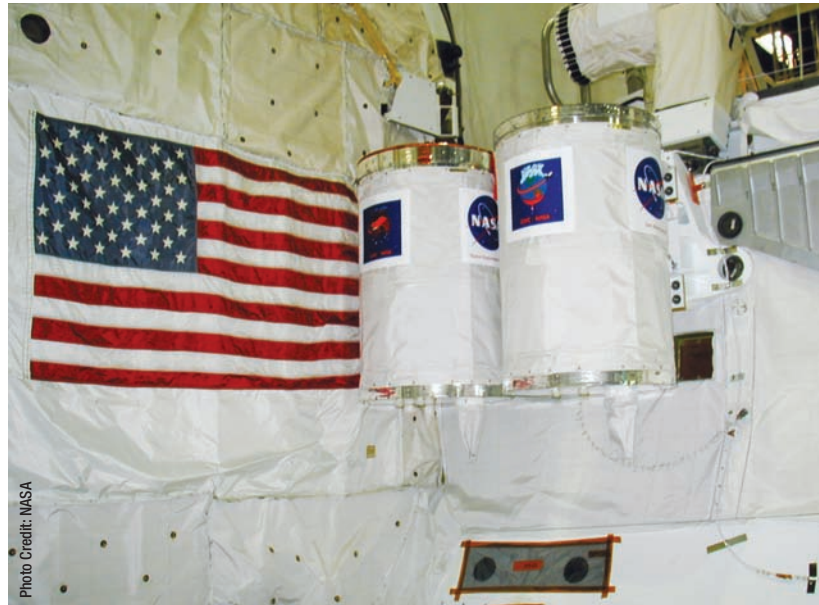
For 19 years, NASA offered flight opportunities to scientists and students with its Getaway Special canisters, which are shown here in the Space Shuttle cargo bay.
