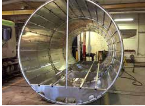
Stringers and aluminum skin installed in Plant Production Module.
