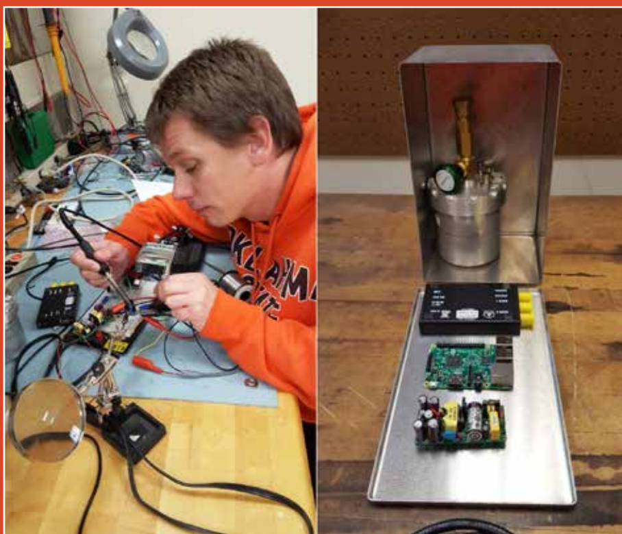
Left: OSU Grad Student Oliver Causey working on the ATED power supply. Right: Detector head (cylindrical canister), spectrometer, computer and power supply with ATED enclosure.
