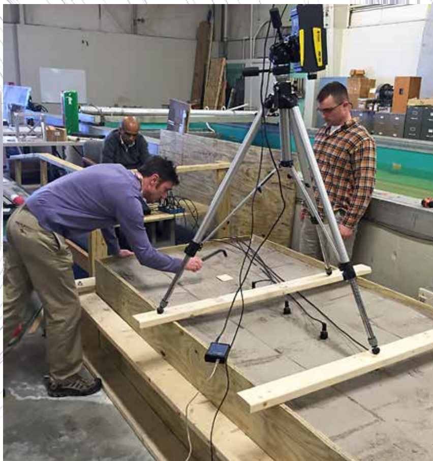
Testing of the laser vibrometer sensing Rayleigh waves in a sand tank. From left to right are Prof. Chris Baxter, Prof. Gopu Potty, and graduate student Tyler Pickering.
