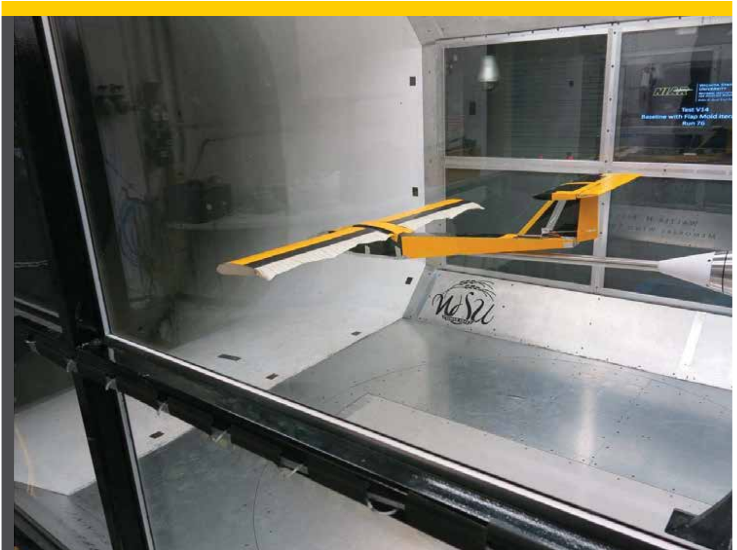
A prototype morphing UAV in the WSU Wind Tunnel.
