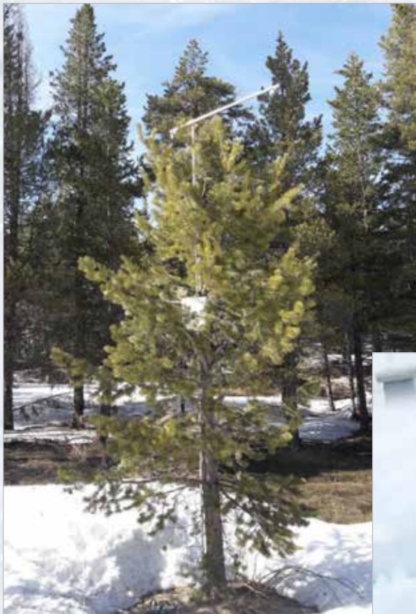
Figure 1. Infrared radiometers were mounted in an isolated tree to measure the surface temperature of the tree and the snow during coincident thermal imagery overflights by a UAS and airplane.
