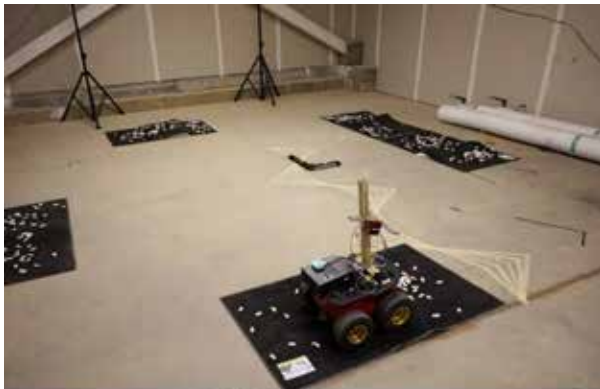
Experimental results: Robot trajectories estimated by the 3 methods on indoor mock terrain (experiment 6). Sand bags are placed on the ground and covered by outdoor mats to create mock terrain.
