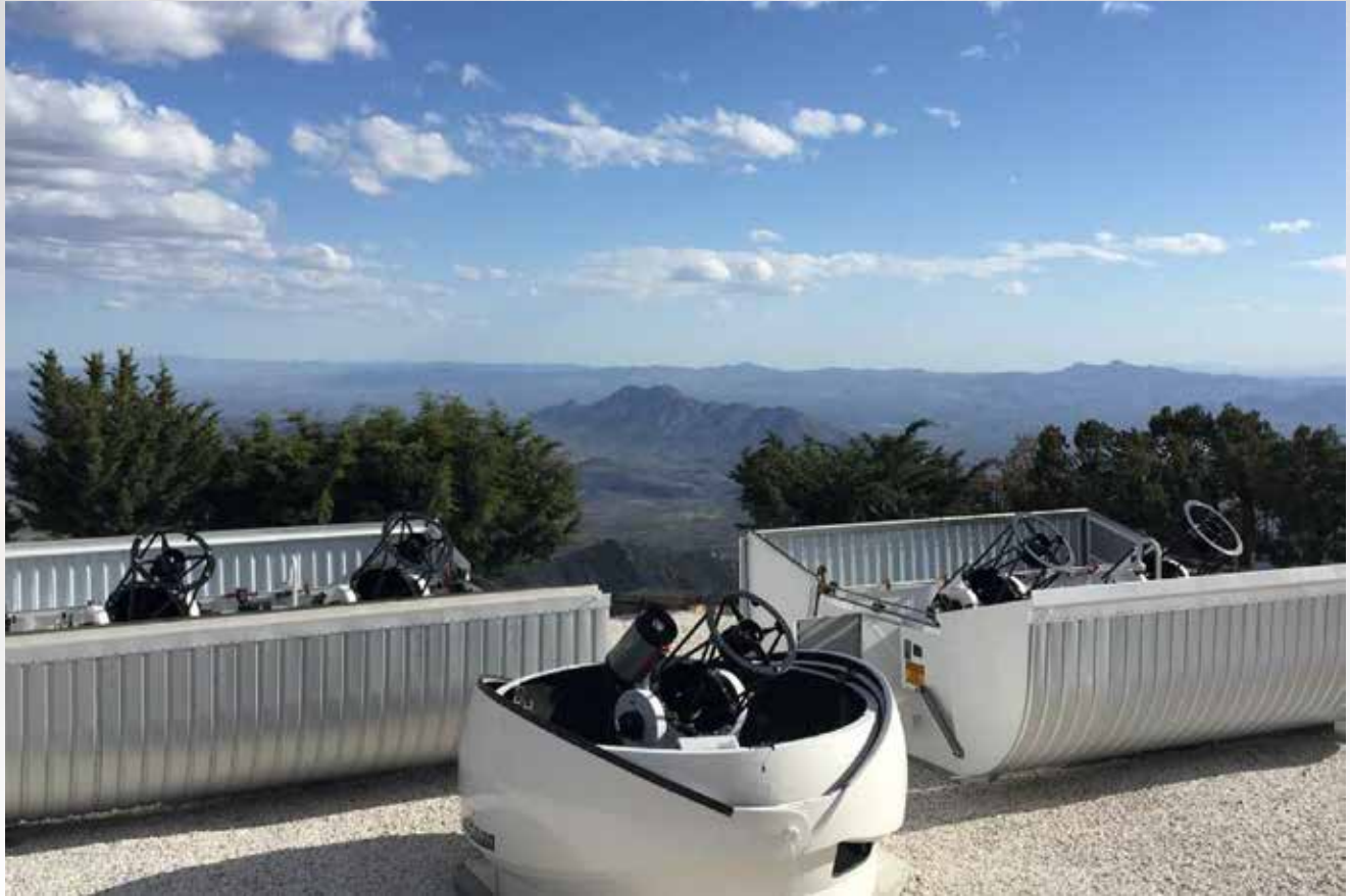
The MINERVA telescopes at Whipple Observatory outside Tucson, Arizona. The University of Montana telescope is second from the right. The MINERVA telescopes can work together by pooling their collected light together or work independently. They are remotely controlled.
