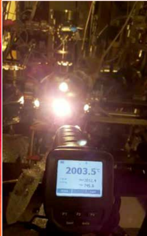
(Left) Tungsten filament heated to 2003.5 °C inside vacuum chamber.
