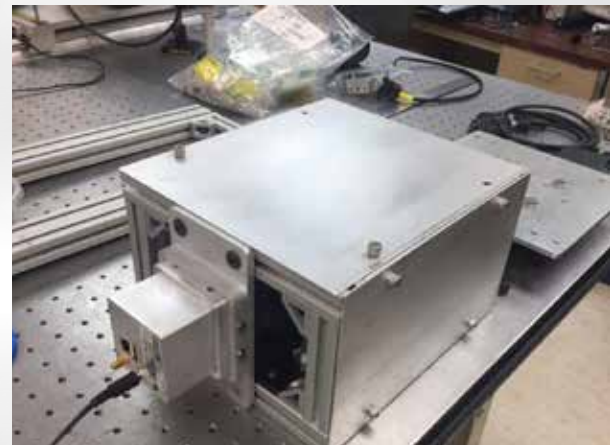
Rear view, with microbolometer visible on left. This photograph shows the uncooled implementation. Here, the interferometer is the same, the only difference being the detector (an uncooled INO mXCam MWIR microbolometer) and imaging lens.
