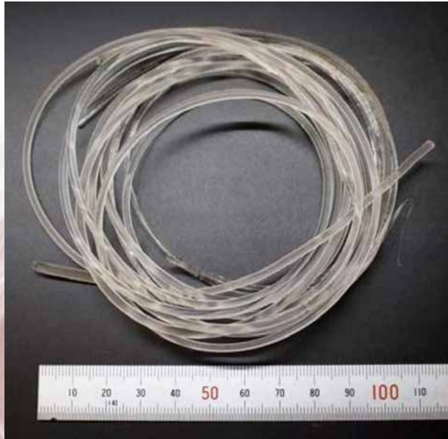
Ionomer precursor pellets drawn into filament.
