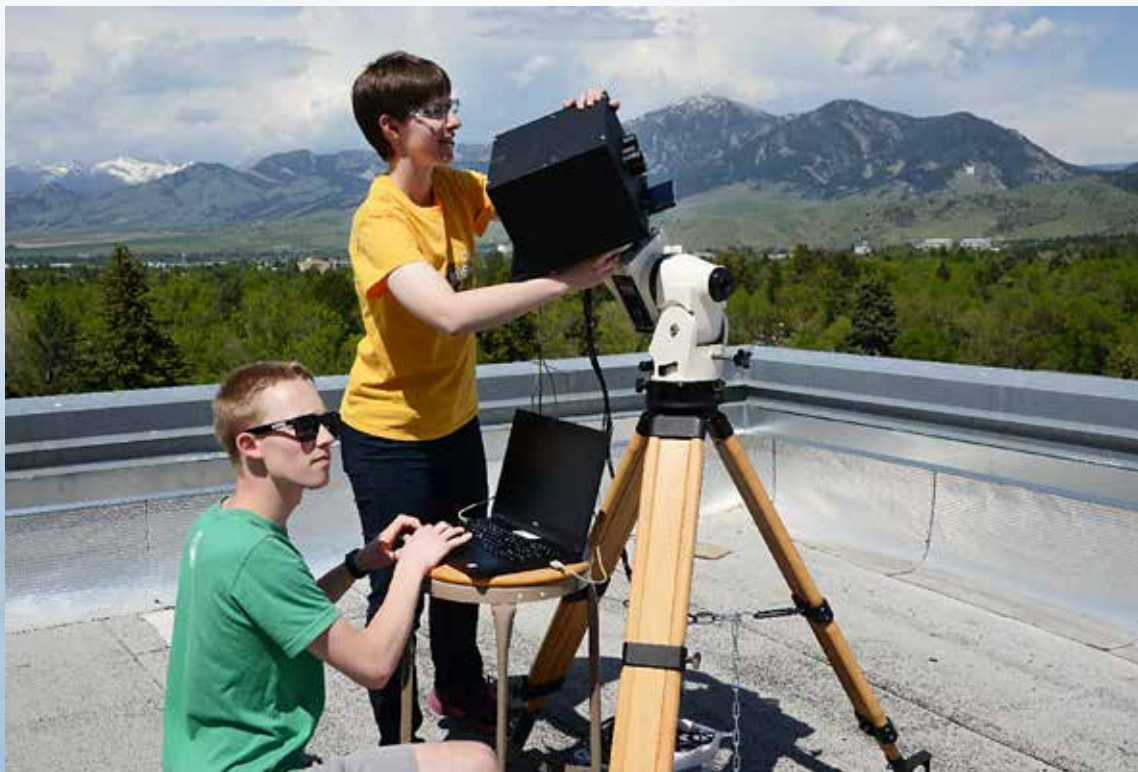
Two recent Electrical Engineering graduates working with the short-wave infrared polarimeter they helped build as their senior project at Montana State University.
