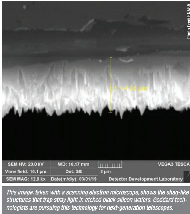
*This image, taken with a scanning electron microscope, shows the shag-like structures that trap stray light in etched black silicon wafers. Goddard technologists are pursuing this technology for next-generation telescopes.*
