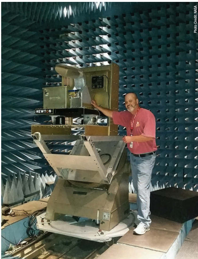
Goddard technician Stephen Seufert stands inside Goddard's Electro-Magnetic Anechoic Chamber, where technicians tested the SWESARR instrument and its unique antenna.
