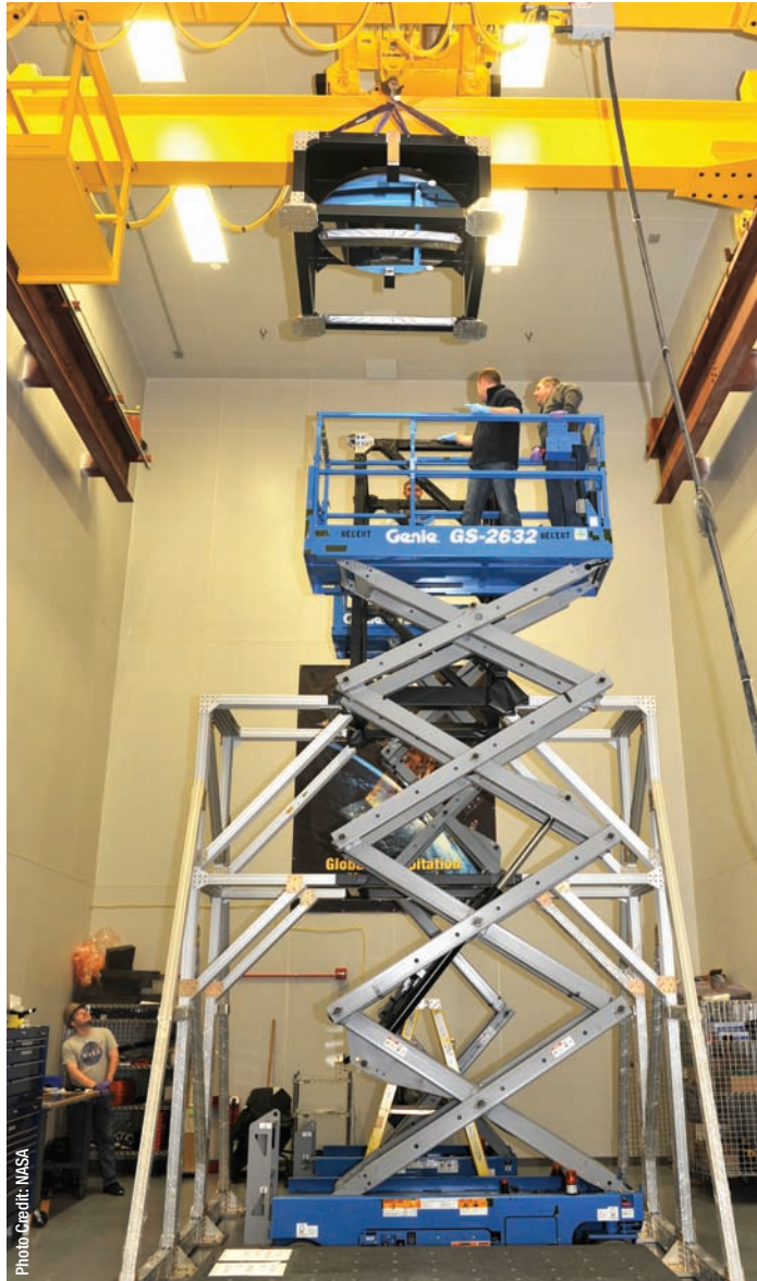
Technicians assemble a new 25-foot test facility, equipped with a 3.3-foot parabolic optical mirror, which will be used to align NICER/SEXTANT's 56 optics and detectors.
