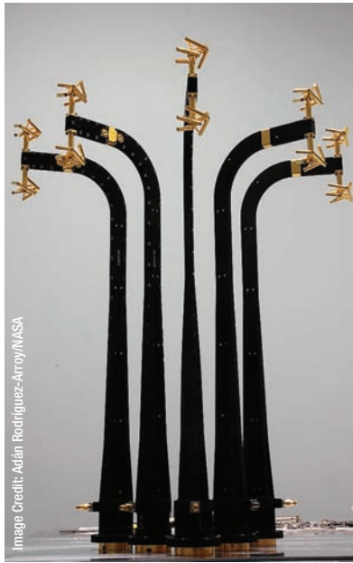
This Goddard-developed S-band communications antenna is one of many enabling technologies on NASA's MMS mission.
