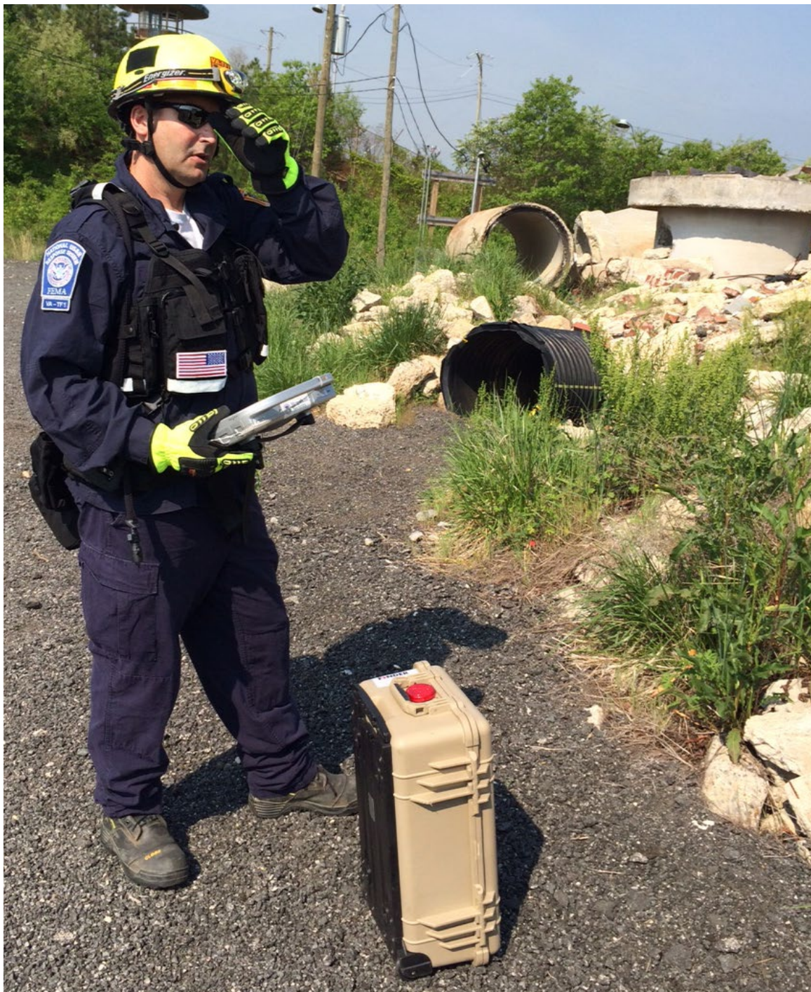
Above: The Finding Individuals for Disaster and Emergency Response (FINDER) prototype technology can locate individuals buried under rubble in disaster scenarios. This photo is from a previous test. Credits: NASA/JPL-Caltech/DHS
