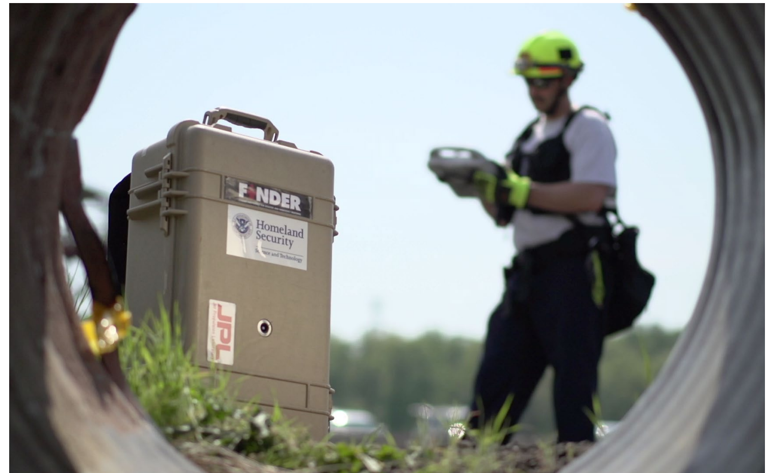
Above: The Finding Individuals for Disaster and Emergency Response (FINDER) prototype technology can locate individuals buried under rubble in disaster scenarios. This photo is from a previous test. Credits: NASA/JPL-Caltech/DHS
