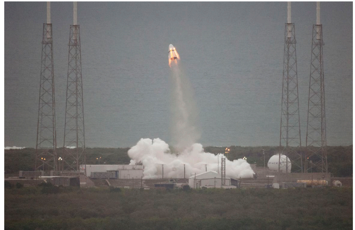
Above: Eight SuperDraco engines boost a SpaceX Crew Dragon spacecraft away from Space Launch Complex 40 at Cape Canaveral Air Force Station in an emergency pad abort simulation. Photo credit: NASA
