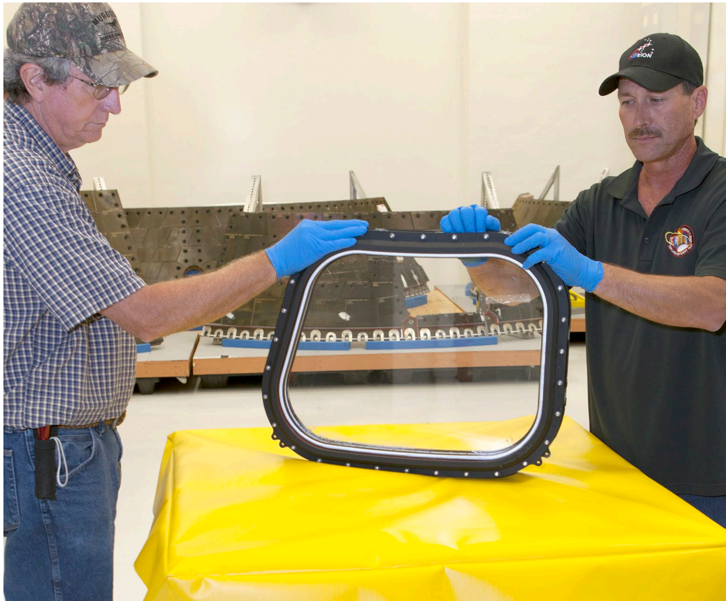
Technicians remove a side thermal window from one of Orion's tile panels inside the Neil Armstrong Operations and Checkout Building high bay at Kennedy Space Center on May 15. The tile panels with thermal windows intact were removed from Orion in the Launch Abort System Facility after the spacecraft returned to Kennedy in late December. All of the windows are being removed and disassembled for post-flight inspection for any signs of micrometeoroid or orbital debris impacts or other potential glass damage. Orion launched aboard a United Launch Alliance Delta IV Heavy rocket on Exploration Flight Test-1 on Dec. 5, 2014. After a two-orbit, 4.5 hour mission, Orion splashed down in the Pacific Ocean and was retrieved by NASA, Lockheed Martin and the U.S. Navy. The spacecraft was secured in the well deck of the USS Anchorage and brought to Naval Base San Diego, where it was offloaded, secured in a container and transported back to Kennedy for analysis. Orion will next launch atop the agency's Space Launch System rocket. The spacecraft will help enable missions to an asteroid and on toward Mars. For more information, visit www.nasa.gov/orion . Photo credit: NASA/Dimitri Gerondidakis
