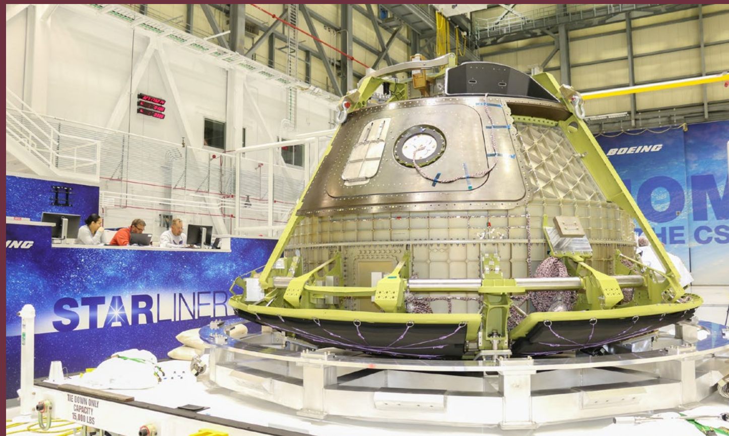
Boeing's Structural Test Article of its CST-100 Starliner spacecraft is readied inside the company's Commercial Crew and Cargo Processing Facility at Kennedy Space Center. Built to the specifications of an operational spacecraft, the STA is intended to be evaluated through a series of thorough testing conditions at facilities in Huntington Beach, California. Photo credit: Boeing
