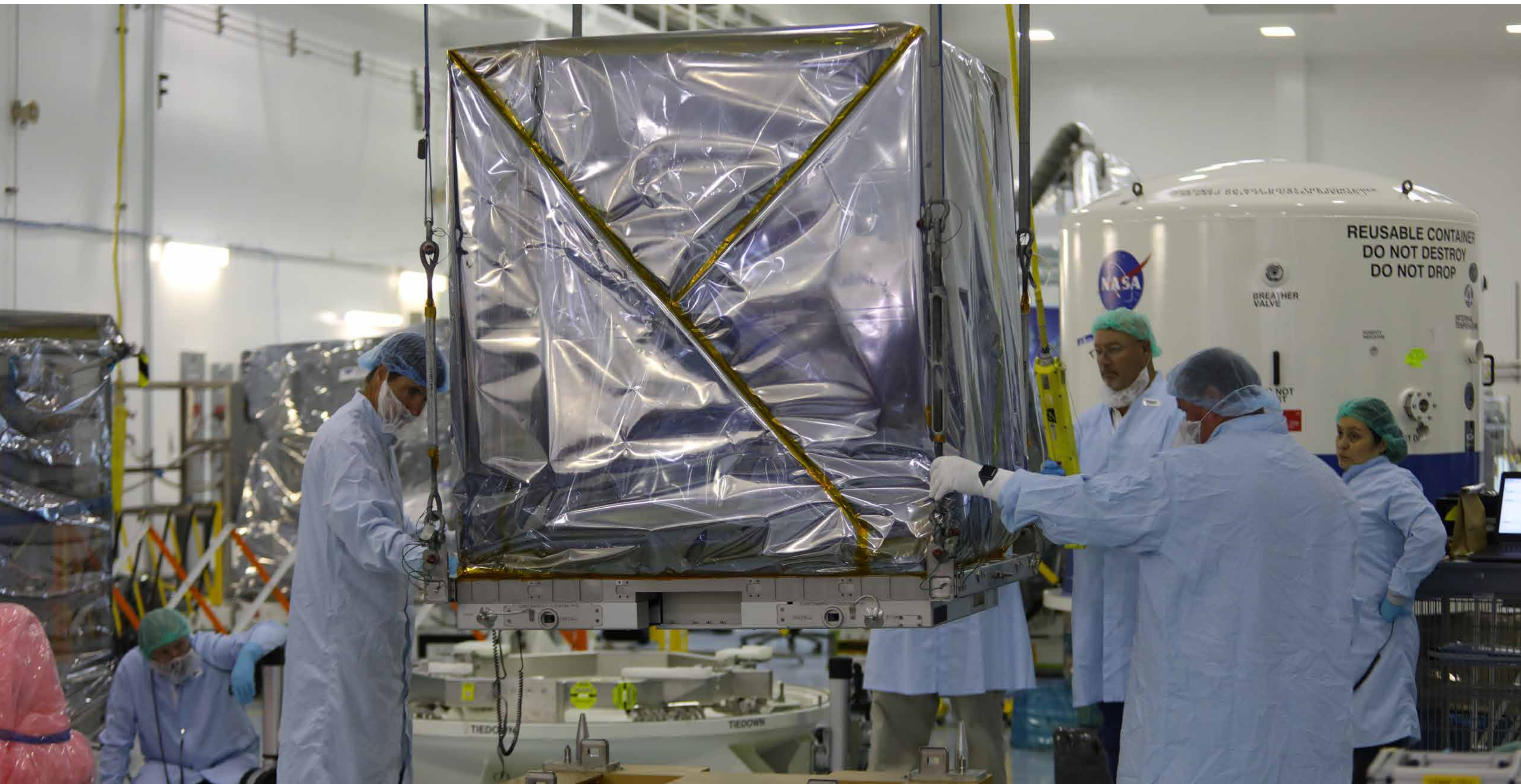
Technicians package the Neutron star Interior Composition Explorer, or NICER, payload April 6 inside the Space Station Processing Facility high bay at Kennedy Space Center. NICER will be delivered to the International Space Station aboard SpaceX's Dragon cargo module, on its eleventh commercial resupply services mission, CRS-11. Photo credit: NASA/Frank Michaux
