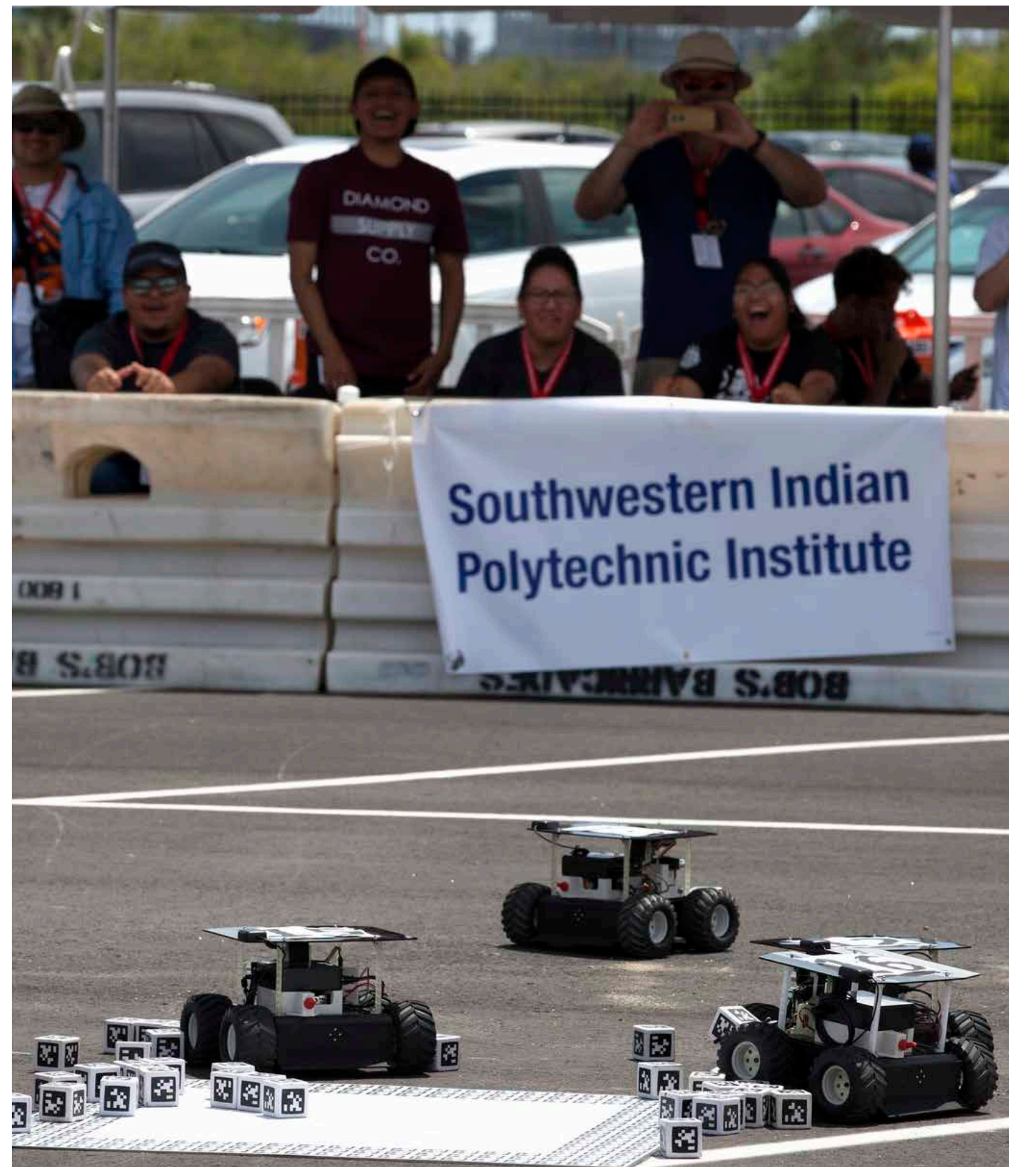
During the final round of the Swarmathon competition at the Kennedy Space Center Visitor Complex, students from Southwestern Indian Polytechnic Institute (SIPI) in Albuquerque, New Mexico, watch their robots as they look for cubes identified by their AprilTags, similar to a barcodes. The Swarmies were programed to deliver the cubes to a "home" square in the middle of a competition arena. SIPI captured first place in the competition winning a $5,000 cash prize. Photo credit: NASA/Kim Shiflett
