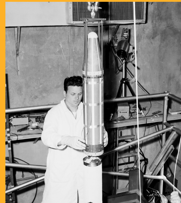
In the gantry at Space Launch Complex 26 at the Cape Canaveral Missile Annex (now Cape Canaveral Air Force Station), a technician lowers the Explorer 1 satellite onto the launch vehicle's fourth stage motor. Photo credit: NASA
