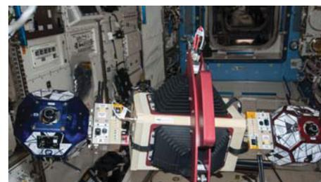
SPHERES-Slosh with tanks partially filled with water conducting a test on ISS
