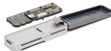
The MinION (Biomolecule Sequencer), a miniaturized DNA sequencer, will enable the first DNA sequencing done in space. Credits: Oxford Nanopore Technologies
