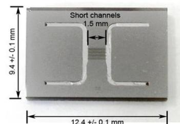
Optical image of the Microchannel Diffusion device.
