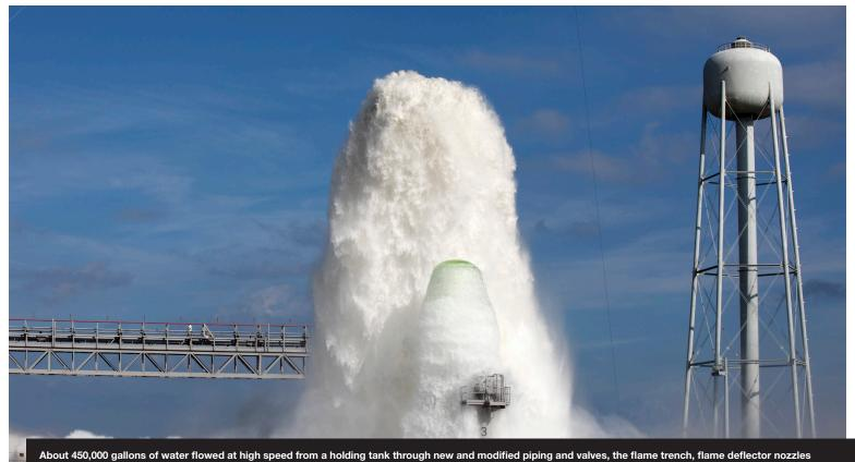
About 450,000 gallons of water flowed at high speed from a holding tank through new and modified piping and valves, the flame trench, flame deflector nozzles and mobile launcher interface risers during a wet flow test at Launch Pad 39B at NASA's Kennedy Space Center in Florida. At peak flow, the water reached about 100 feet in the air above the pad surface. Photo credit: NASA/Kim Shiflett
