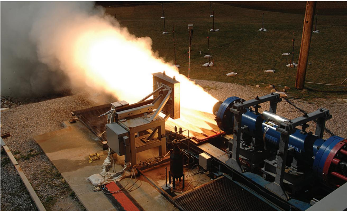
Marshall tested a small solid rocket motor designed to mimic NASA's SLS booster. The test provided an effective way to evaluate a new nozzle insulation material.
