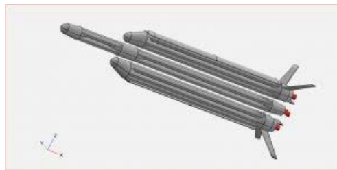
Figure 10.42: Austral Launch Vehicle Concept. Image courtesy of Heliq Advanced Engineering.
