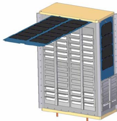
Figure 7.4: Passive Thermal Louver on 6U CubeSat Dellinger. Image Courtesy NASA Goddard (2015).
