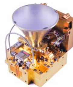
Figure 9.12: Ka-band transmitter with a horn antenna. Image courtesy of Astro Digital.
