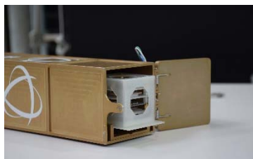
Figure 10.35: Albapod holding 2P PocketQube. Image courtesy of Alba Orbital.
