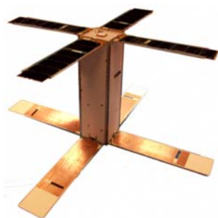
Figure 9.5: SNaP spacecraft with Haigh-Farr's deployable UHF Crossed Dipole antenna. Image courtesy of Haigh.
