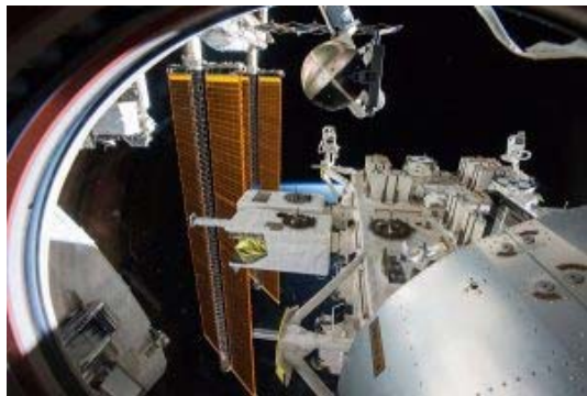
Figure 4.8: Module of DSSP thrusters. Image courtesy of Nicholas et al. (2013).
