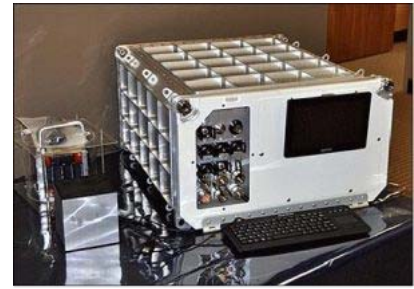
Figure 10.19: NanoRacks Platform 3 image with centrifuge housing. Image courtesy of Nanoracks.
