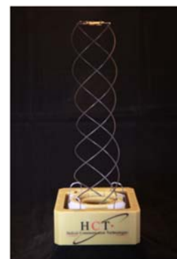
Figure 9.6: Example of deployable quadrifilar helical antenna. Image courtesy of Helical Communication Technologies.
