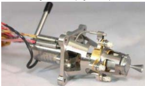
Figure 4.2: GR1 thruster. Image courtesy of Masse et al. (2015).
