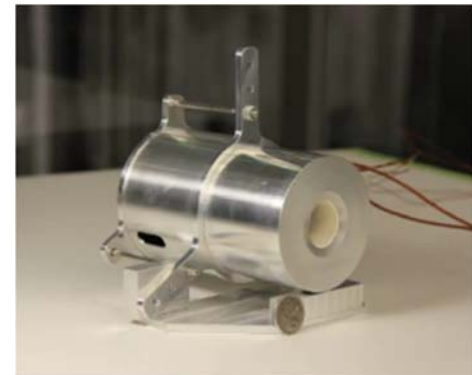
Figure 4.17: Cylindrical Hall Effect Thruster. Image courtesy of UTIAS SFL.
