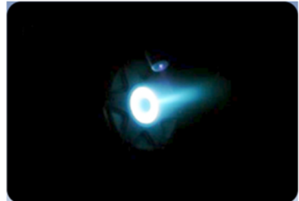
Figure 4.16: BHT-200 during operation. Image courtesy of Busek Co Inc.
