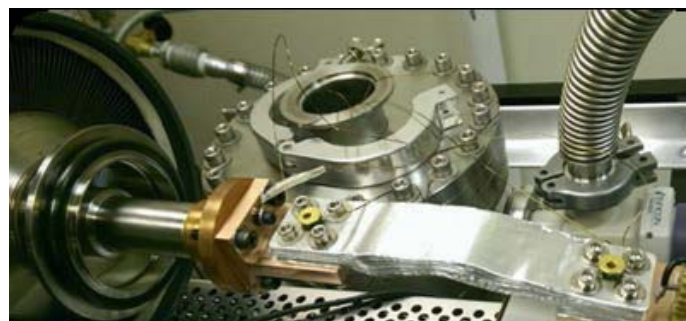
Figure 7.2: Thermal Management Technologies Aluminum thermal strap test. Image Courtesy of Thermal Management Technologies (2015).
