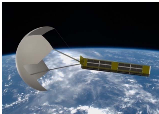
Figure 12.4: Deployment of the Exo-Brake device. Image courtesy of F.A.Tanner.
