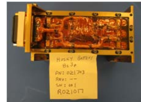
Figure 3.11: ABSL COTS Li-ion Battery. Image courtesy of ABSL (2007).
