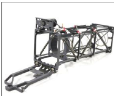
Figure 10.29: Tyvak 6U Rail-POD Dispenser. Image courtesy of Tyvak Nano-Satellite Systems LLC.
