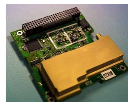
Figure 9.8: CubeSat-compatible S-band transmitter, to be used with either amateur or commercial bands. Image courtesy of AAC-Clyde.
