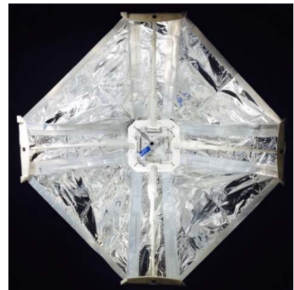
Figure 7.1: End view of Sunshield on CryoCube-1 developed at Sierra Lobo. Image courtesy of Sierra Lobo (2014).
