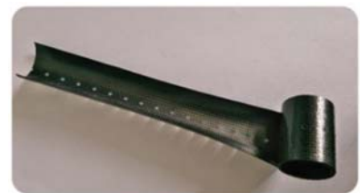
Figure 6.9: The flexible composite member that is employed on the AstroTube. Courtesy of Revels, et al.
