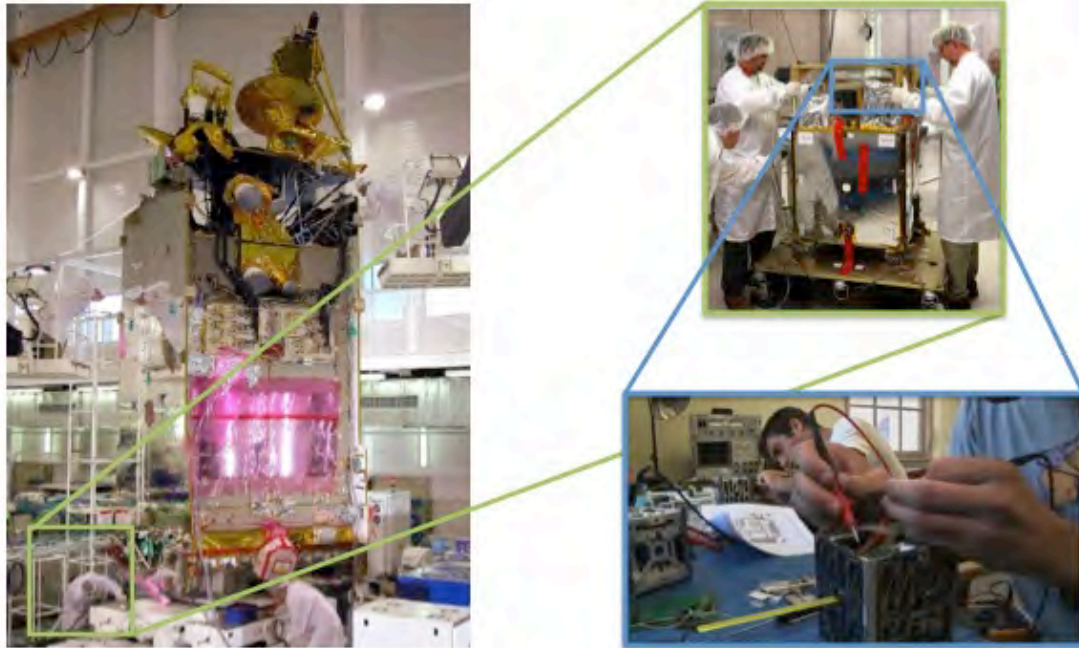
Figure 4: Integration of various spacecraft. (Left) large spacecraft clean room (Intelsat 10-02, image credit: EADS Astrium); (Right) Integration environments for small spacecraft FASTSAT (Top) and Phonesat (Bottom). The blue and green rectangles highlight the differences in size compared to Intelsat 10-02.
