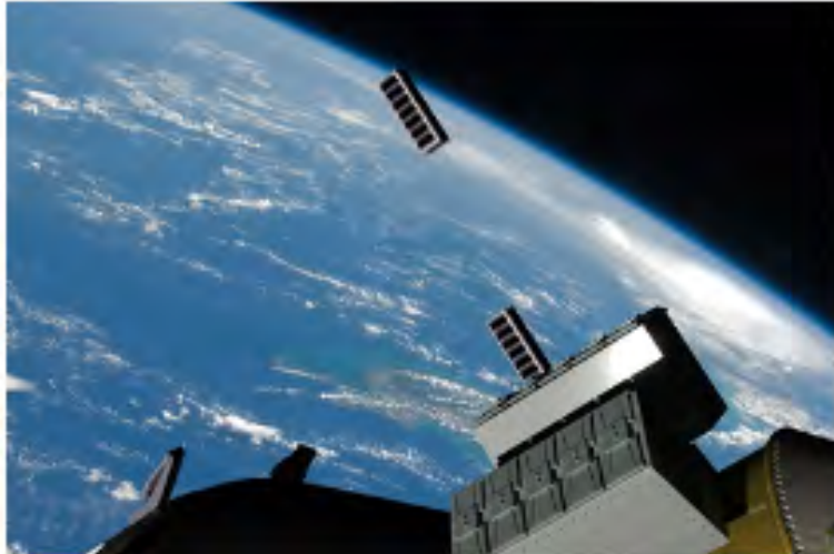
Figure 56: Spaceflight Services depiction of Smallsat ejections from dispenser in low-Earth orbit (LEO) ( Spaceflight Services LLC , 2013).
