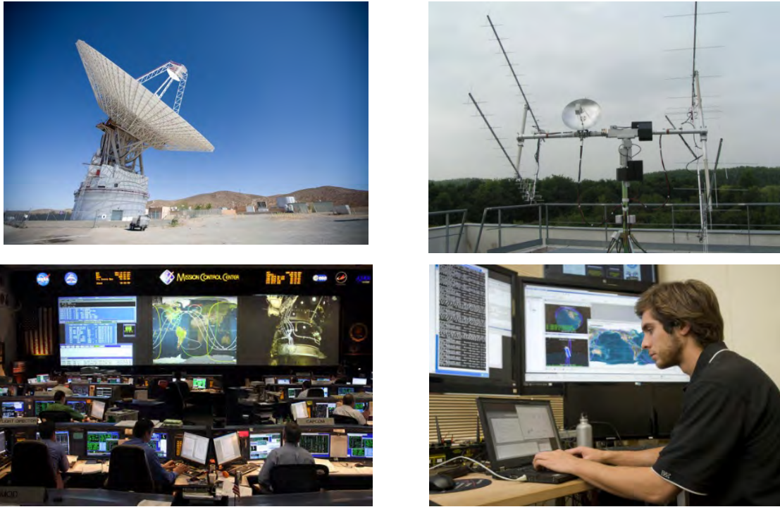
Figure 64: Differences in size and scope between large (left-hand side) and small spacecraft ground systems (right-hand side). Top left: NASA's Deep Space Network (DSN) ground station in Goldstone, CA. Top right: GENSO roof-top ground station at the International Space University, Strasbourg, France. Bottom left: NASA MCC at JSC, Houston, TX. Bottom right: Student operating the small spacecraft MCC at the University of Santa Clara, CA.
