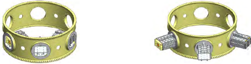
Figure 56: (Left) ESPA SUM with interior mounted CubeSats and (right) exterior mounted (Marin, n.d.).
