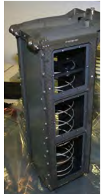
Figure 54: P-POD ejection spring (Image credit: http://rjwagner49.com/Personal/Work/Mayflower/ ).
