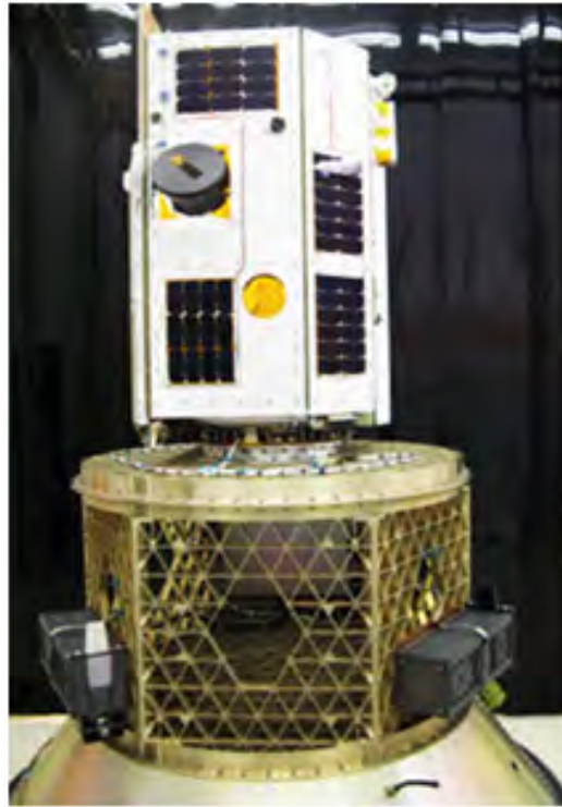
Figure 59: Example of primary payload integrated with smallsat secondary payloads stowed in dispenser (TriSept Corporation, 2013).
