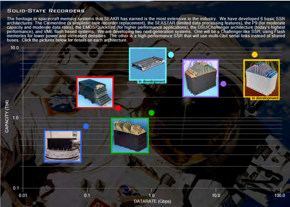
Figure 49: An example of SoA solid state recorder capability (SEAKR).
