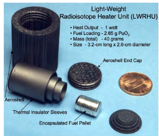
Figure 8: Light Weight Radioisotope Heater Unit compared to the size of a U.S. one cent penny (Image credit: LANL, found in Cataldo, et al., 2011).
