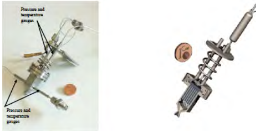
Figure 14: Miniature hydrogen peroxide thruster (Scharlemann, et al., 2011).
