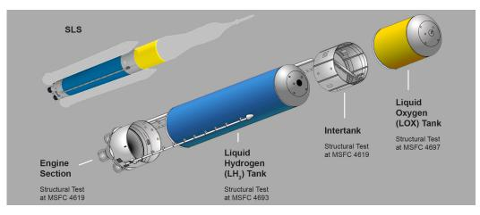
An expanded view of the core stage for NASA's Space Launch System, shows the position of the liquid oxygen and liquid hydrogen tanks that will be tested in the new structural test stands 4693 and 4697 at Marshall.
