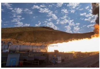
NASA and Northrop Grumman have successfully completed three full-scale development and two full-scale qualification test firings of the five-segment solid rocket motor, as well as the important booster critical design review.
