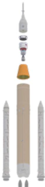
The SLS Block I configuration will be used for NASA's first three Artemis missions. The [Integrated Spacecraft/Payload Element](#) for the SLS Block I crew configuration is located above the core stage and below the Orion spacecraft. It includes elements for in-space propulsion, adapters, and a separation system.
