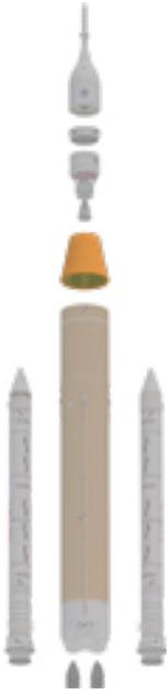
The cone-shaped [launch vehicle stage adapter](#) partially encloses the ICPS and provides the interface between the 27.6-ft. (8.4 m)-diameter core stage and 16.7-ft. (5.1 m)-diameter ICPS. The adapter is 27.5 ft. (8.4 m) tall. Hatches in the adapter allow technicians access to the ICPS during processing at Kennedy. The launch vehicle stage adapter also protects avionics and electrical devices in the ICPS from extreme vibration and acoustic conditions during launch and ascent.
