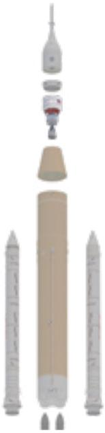
The 45-ft. (13.7 m)-tall, 16.7-ft. (5.1 m) -diameter ICPS is a modified Delta Cryogenic Second Stage, a proven upper stage used on ULA's Delta IV family of launch vehicles. ULA builds the ICPS at its rocket factory in Decatur, Alabama. After completion, it's shipped to ULA's Delta Operations Center at Cape Canaveral Space Force Station on ULA's R/S Rocketship cargo ship for final checkout prior to stacking in the Vehicle Assembly Building.
