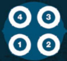
Shown here from the bottom, looking up at the rocket from below, four liquid hydrogen (**LH2**) and liquid oxygen (**LOX**)-fueled **RS-25 ENGINES** are arranged in a square pattern, like legs on a table, providing stability and even distribution of propulsion forces to the rocket. At launch, they will produce
