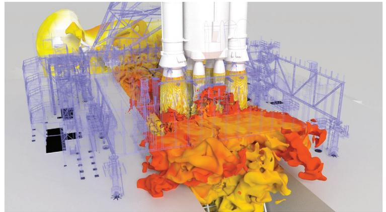
*Ames produced a visualization of SLS exhaust gas flow during liftoff from Launch Complex 39B to accurately understand how liquid and gases flowing during launch can cause various kinds of waves at the launch pad.*
