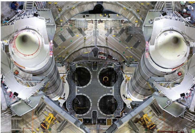
Birds-eye view of the Artemis I solid rocket boosters, the first element to be stacked on the mobile launcher in the Vehicle Assembly Building, awaiting the core stage.
