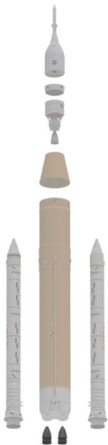
Four **RS-25 engines** power SLS for its eight-minute climb to Earth orbit, together with a pair of solid rocket boosters that operate for the first two minutes of ascent. The RS-25 is formerly known as the Space Shuttle Main Engine (SSME). It flew successfully on 135 space shuttle missions.
