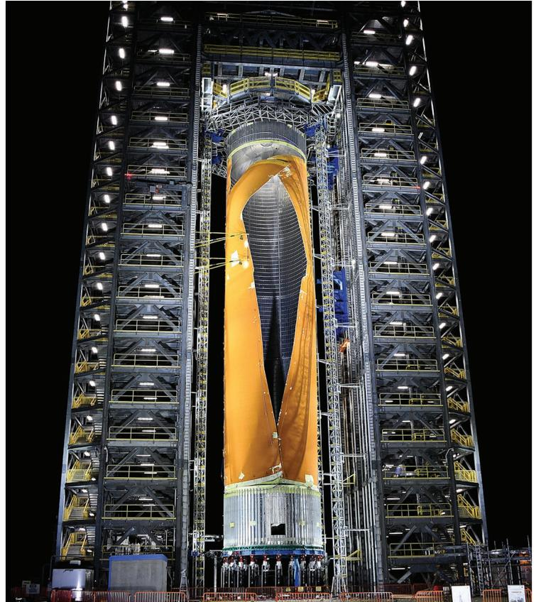
*The test version of the SLS liquid hydrogen tank withstood more than 260 percent of expected flight loads over five hours before it buckled, then ruptured, giving engineers real-world data to reinforce computer models.*
