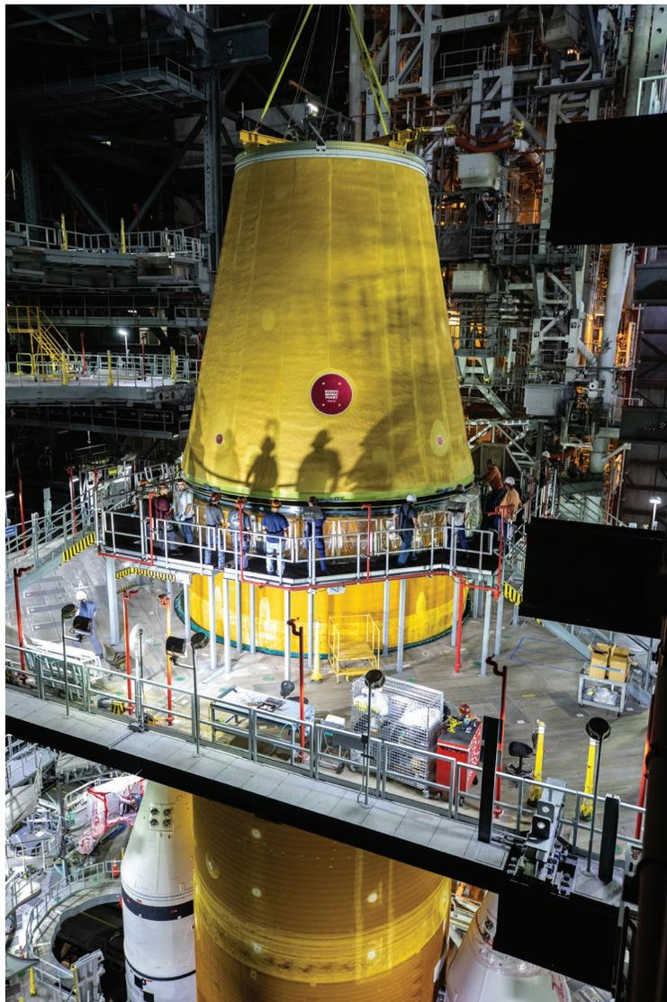
*Teledyne Brown Engineering is the lead contractor for the launch vehicle stage adapter that has a pneumatically activated frangible joint that separates it and the core stage from the ICPS, Orion stage adapter, and Orion during flight.*
