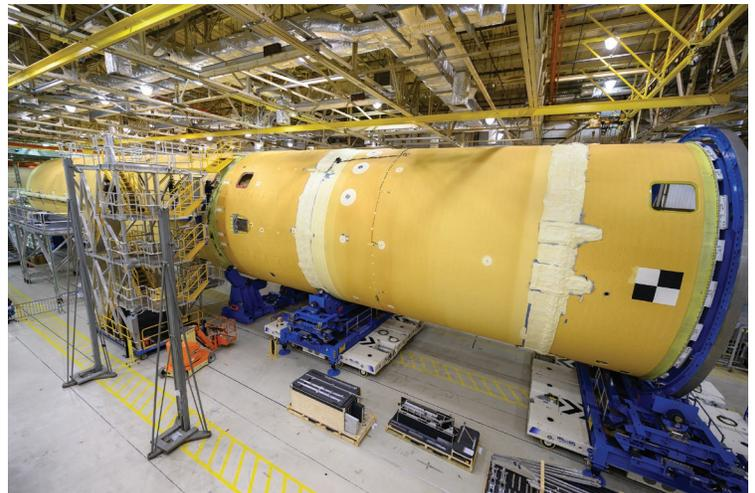
Connecting feedlines and other external components to the fully assembled Artemis I core stage at Michoud.
