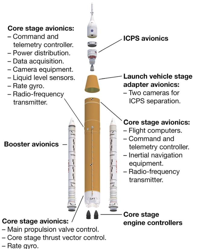
Avionics throughout the elements of SLS monitor the rocket's health and control the flight.
