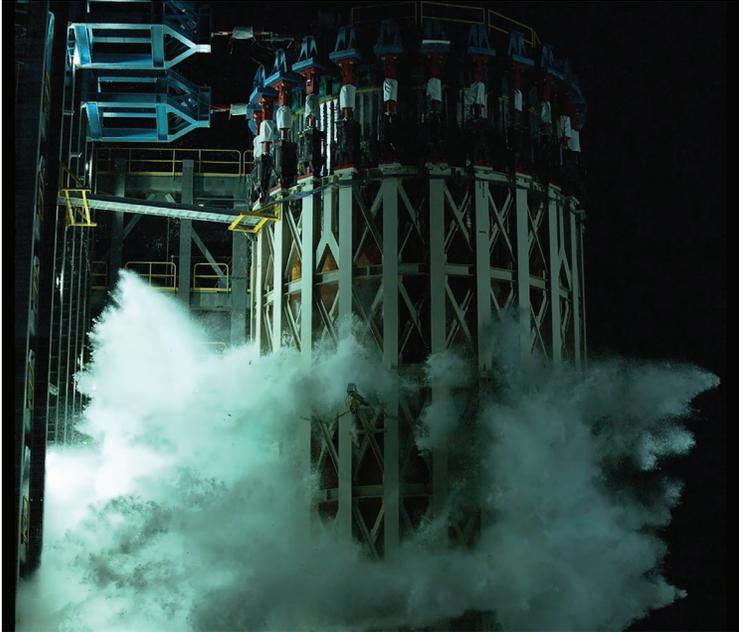
*Hydraulic cylinders applied millions of pounds of force to the liquid oxygen tank test article, completing 20 tests until it failed, providing engineers with valuable data on the tank's structural capabilities.*
