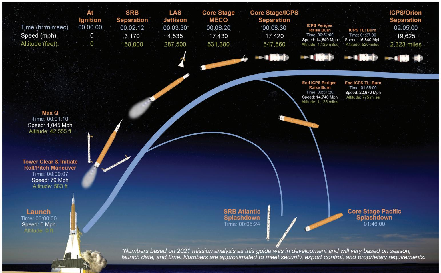
Major events of the Artemis I flight, including solid rocket booster jettison, core stage and launch vehicle stage adapter separation, and ICPS and Orion stage adapter separation from Orion. Following separation with Orion, CubeSat payloads will be released into deep space.
