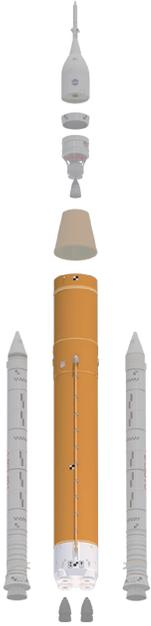
The SLS **core stage** is the tallest rocket stage NASA has ever built. It measures approximately 212 ft. (64.6 m) tall and 27.6 ft. (8.4 m) in diameter (excluding thermal protection system foam and flanges). Its fully fueled weight, excluding engines, is 2.4 million lbs. (1,090 t).
