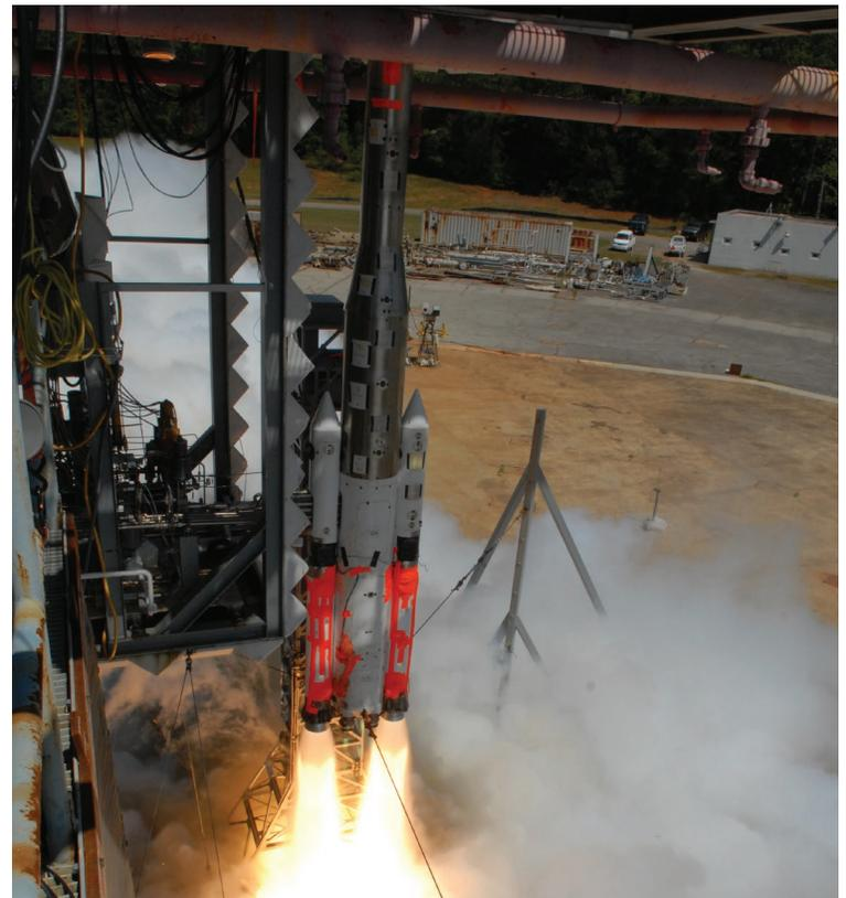
*A five-percent scale model of SLS undergoes acoustic testing in 2014 at Marshall.*
