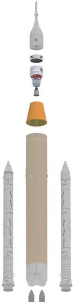
The SLS Block I configuration will be used for NASA's first three Artemis missions. The [Integrated Spacecraft/Payload Element](#) for the SLS Block I crew configuration is located above the core stage and below the Orion spacecraft. It includes elements for in-space propulsion, adapters, and a separation system.
