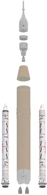
A pair of **solid rocket boosters** attached to the core stage supply more than 75 percent of total SLS thrust for the first two minutes of flight, operating with the four RS-25 main engines. Based on the space shuttle solid rocket boosters, the SLS boosters are the largest, most powerful solid propellant boosters ever built for flight. Each SLS booster is 177 ft. (54.1 m) tall, 12 ft. (3.7 m) in diameter, and weighs 1.6 million lbs. (726 t) when filled with solid propellant.
