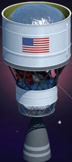
THE INTERIM CRYOGENIC PROPULSION STAGE WILL BE POWERED BY AN AEROJET ROCKETDYNE RL10B-2 ENGINE, PRODUCING **24,750 POUNDS OF MAX THRUST.**
