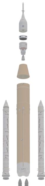
The highest SLS element in the SLS stack, the [Orion stage adapter](#), connects the ICPS to the Orion spacecraft. The Orion stage adapter is 18 ft. (5.5 m) in diameter, 5 ft. (1.5 m) tall, and is made of lightweight aluminum.
