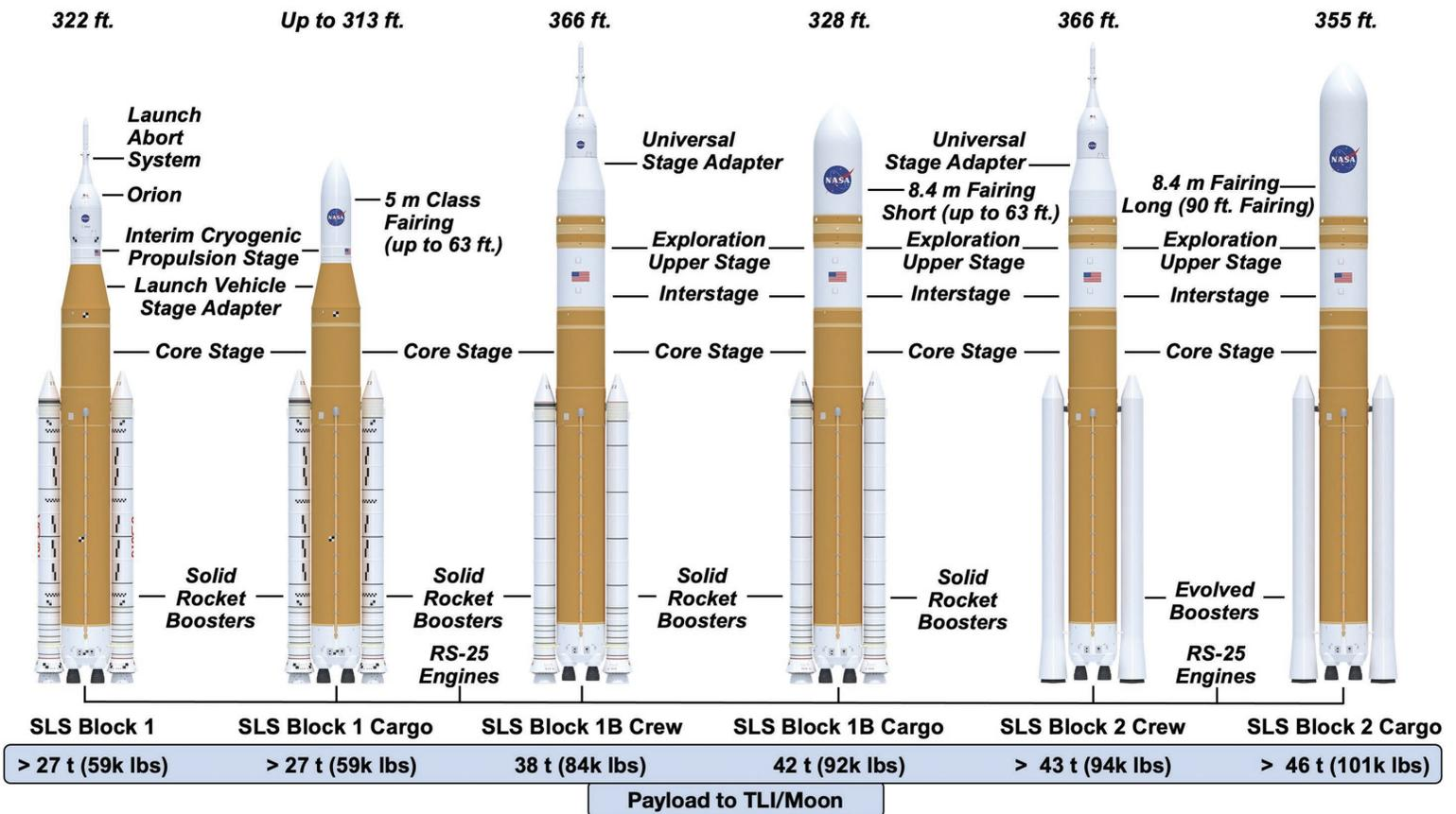
SLS Block 1 with an uncrewed Orion will launch the Artemis I mission. Following the first three Artemis missions, SLS will evolve to a more powerful Block 1B configuration with a new Exploration Upper Stage replacing the ICPS. The ultimate variant, Block 2, will incorporate evolved boosters to increase payload mass to TLI to at least 101,000 lbs. (46 t).
