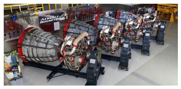
Four RS-25 engines that will power the Space Launch System. (Aerojet Rocketdyne/NASA)
