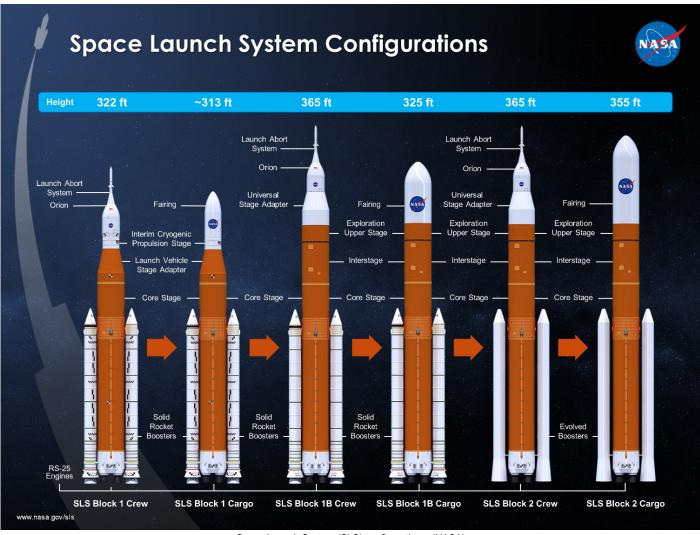
Space Launch System (SLS) configurations. (NASA)
