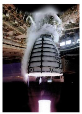
RS-25 engine undergoing a hot-fire test. (NASA)
