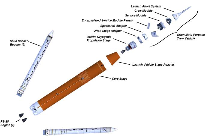
Initial Block 1 Configuration Concept for the Space Launch System. (NASA)
