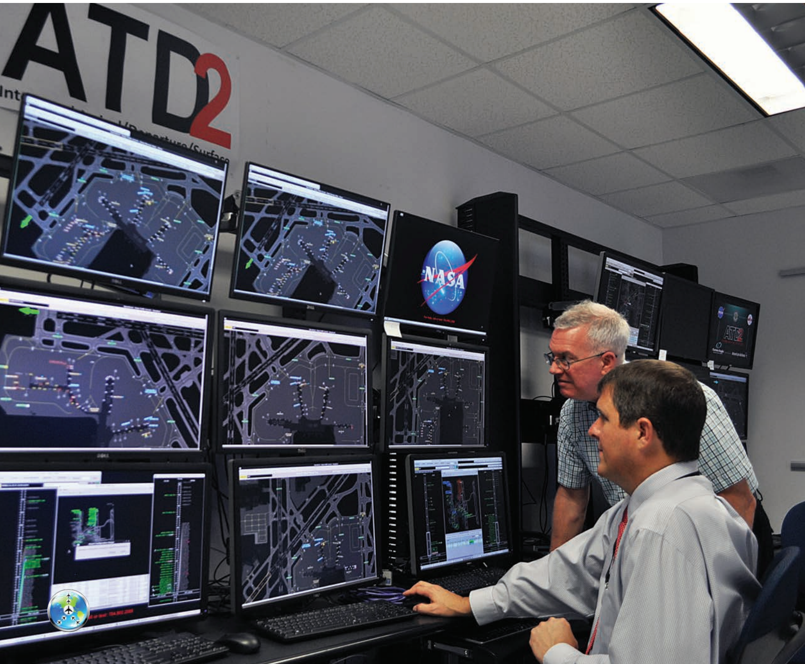
At NASA's air traffic management laboratory near the Dallas/Ft. Worth International Airport in Texas, researchers Al Capps (seated) and Paul Borchers demonstrate Airspace Technology Demonstration 2 tools that air traffic managers have been successfully testing since 2017 at the Charlotte Douglas International Airport in North Carolina to more efficiently direct departing traffic. Image credit: NASA / Jim Banke
