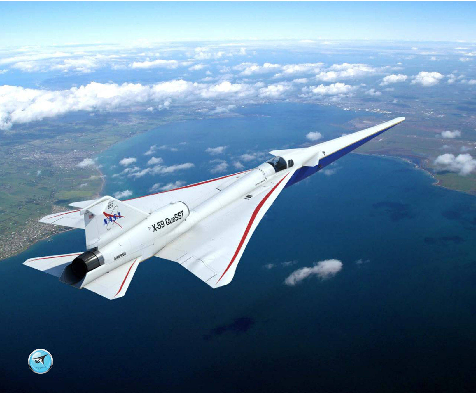
NASA's X-59 QueSST, an experimental piloted aircraft designed to fly faster than sound without producing the annoying – if not alarming – sonic booms of previous supersonic aircraft is taking shape. Image credit: Lockheed Martin
