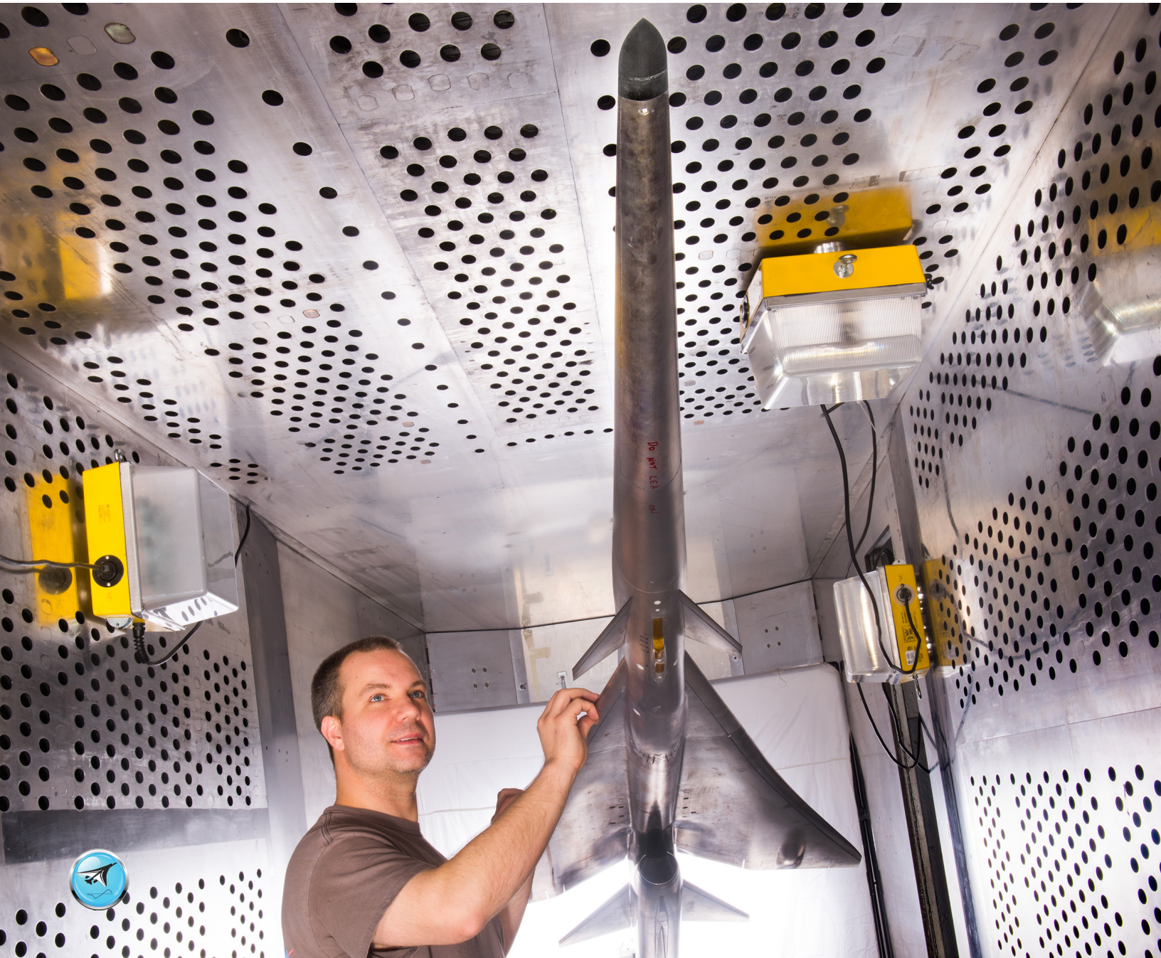
Mechanical technician Dan Pitts prepares a nine percent scale model of Lockheed Martin's Quiet Supersonic Technology (QueSST) X-plane preliminary design for its first high-speed wind tunnel tests at NASA's Glenn Research Center. Image credit: NASA
