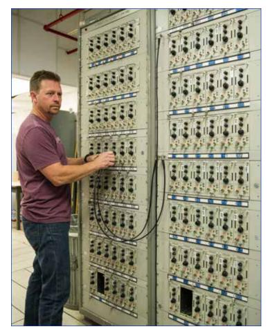
(Bottom left photo) Lockheed Martin Test Operation Contract employee Scotty Herrin checks the status of the A-1 Test Stand accelerometer, which measures rocket engine pump vibrations during a test.
