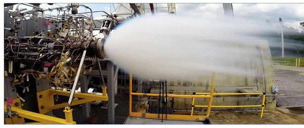
Operators at the E-2 Test Stand at Stennis conduct a test of the oxygen preburner component being developed by SpaceX for its Raptor rocket engine, which is being built to power flights to Mars
