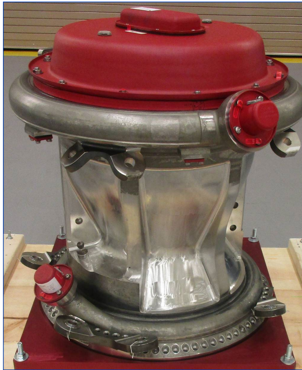
NASA is testing a new main combustion chamber made by modern manufacturing techniques during RS-25 engine hot fires at Stennis.
