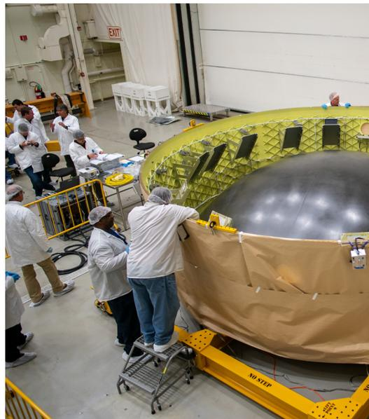
*The completed Orion stage adapter for the SLS rocket for the Artemis I flight, with the mounting brackets for CubeSats in their dispensers.*
